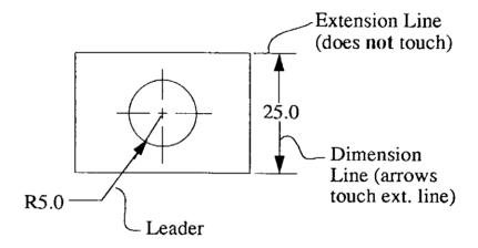
Feature: a geometric shape or entity on the object (i.e. an edge, a cylinder,...)
