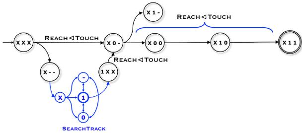
Fig. 9. This diagram shows the transition diagram for the policy learned for REACHTOUCH after 25 episodes. The state vector is  $\mathbf{s} = (p_{st} \text{ Preach } p_{touch})$  where  $p_{st}$  is the state value of the SEARCHTRACK program. The hierarchical use of SEARCHTRACK is indicated by the abstract transition icon introduced in Figure 5.
