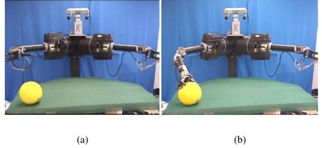
Fig. 3. Frames (a) and (b) show the robot before and after reaching to a highly-saturated object with its right arm.
