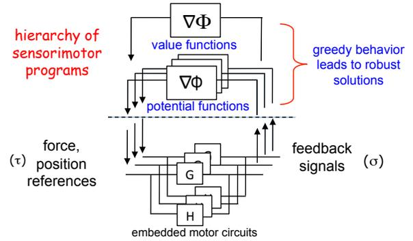
Fig. 2. The hierarchical control basis architecture. Control actions descend potential functions by submitting reference inputs to lower-levels and ultimately, to embedded motor circuits.  $H$  and  $G$  represent feedback and feedforward transfer functions, respectively.
