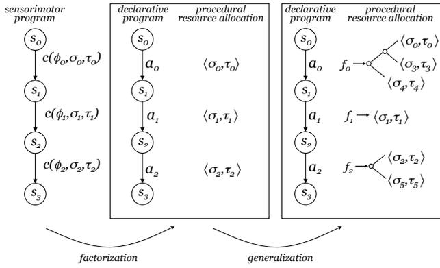
Fig. 12. Sensorimotor programs in the control basis can be factored into procedural and declarative components and generalized to new environmental contexts, by means of the policy  $\psi(a_i, f_j)$ , where  $a_i \in \mathcal{A}$  and  $f_j \in \mathcal{F}$ .
