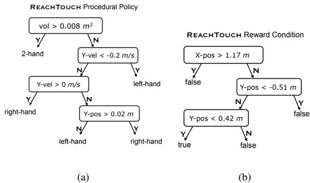
Fig. 13. The decision tree in (a) shows the resulting procedural policy for choosing which arm to allocate for reaching based on object volume, position, and velocity. The tree in (b) shows conditions under which REACHTOUCH is likely to achieve reward. It captures when objects are out of the robot’s work space in terms of their position.
