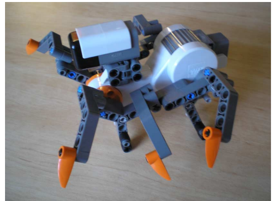
Fig. 17. An “Ant” robot using the Lego Mindstorms NXT platform. This robot has one motor controlling all legs and an accelerometer. Image from [30].
