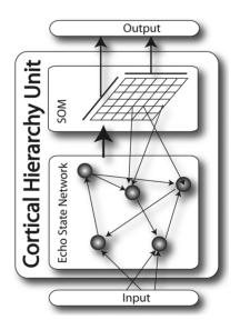
Fig. 7. Abstract model of a cortical microcircuit. Input perturbs an ESN reservoir, which is then read by a SOM. The SOM also provides an input to the ESN and the location of the winning SOM unit in SOM space is provided as the output of the unit.
