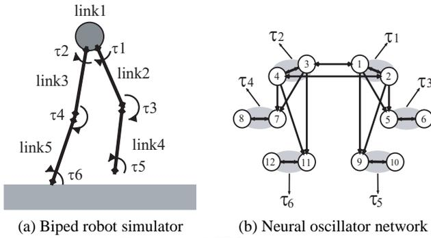
Figure 4: Structure of CPG-driven biped robot
