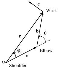
FIGURE 1. Arm configuration or posture is described by a set of relative position vectors  $\mathbf{a}, \mathbf{b}, \mathbf{c}$  relating the joints. The position of a joint is defined to be its center of rotation. The vector  $\mathbf{a}$  designates the position of the elbow relative to the shoulder;  $\mathbf{b}$  designates the position of the wrist relative to the elbow;  $\mathbf{c}$  designates the position of any point in the hand relative to the wrist.
