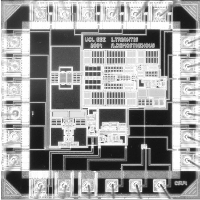
Fig. 10. Chip microphotograph.
