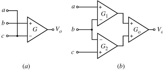
Fig. 2. Tripolar ENG amplifier configurations. (a) Quasi-tripole (QT). (b) True-tripole (TT).
