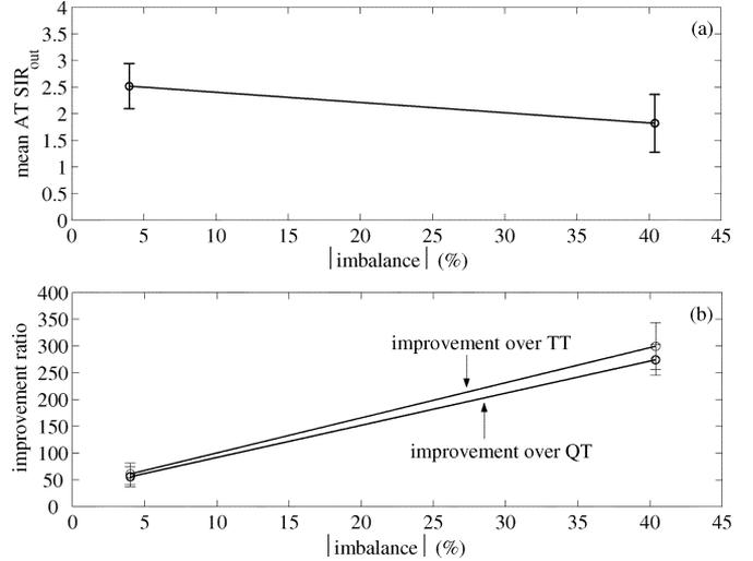
Fig. 15. (a) Mean AT  $SIR_{out}$  versus (absolute) imbalance for all 20 chips. (b)  $SIR_{out}$  improvement over the ideal TT and QT counterparts versus (absolute) imbalance.
