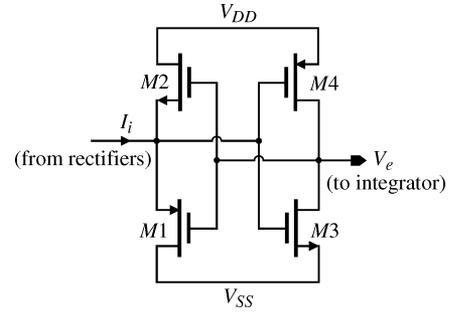
Fig. 7. Comparator circuit.
