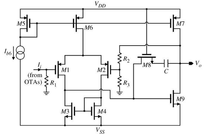
Fig. 9. Output-stage amplifier circuit.
