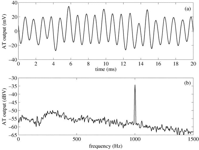
Fig. 13. System output for +20% imbalance. (a) Time-domain. (b) Frequency-domain.
