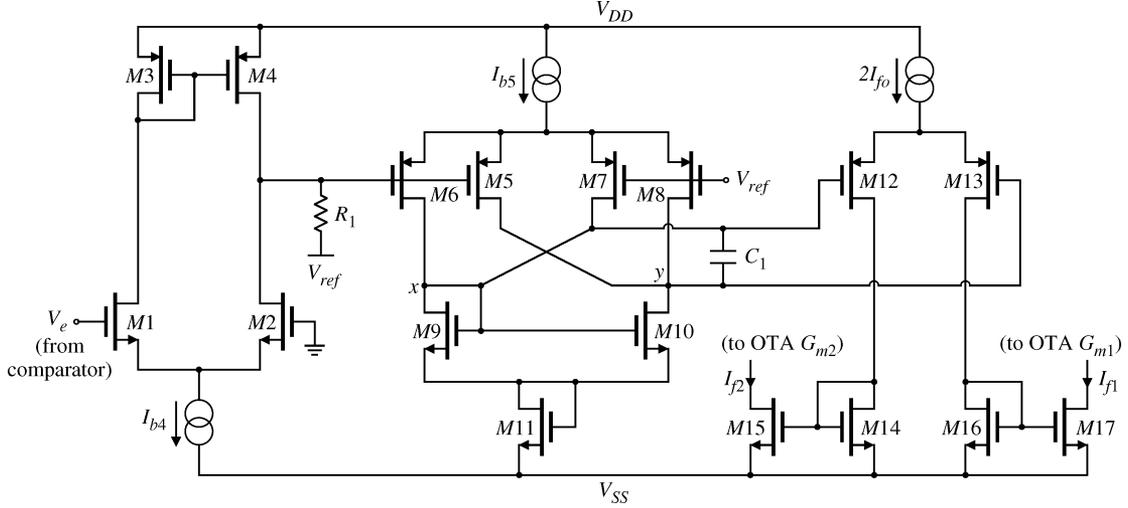
Fig. 8. Large time-constant integrator circuit.
