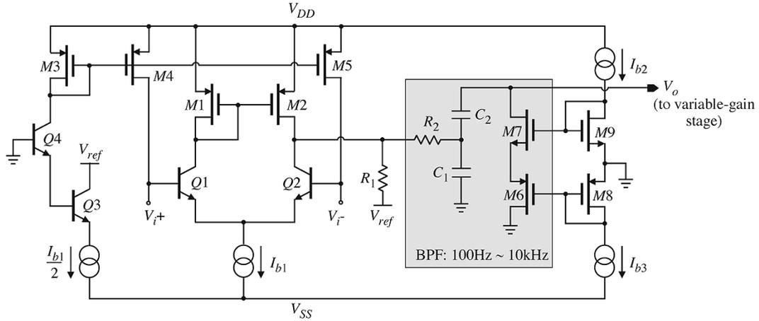
Fig. 4. Preamplifier circuit.
