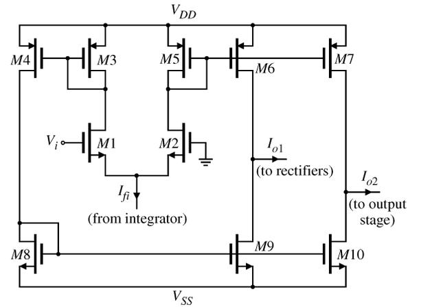
Fig. 5. Variable-gain OTA circuit.
