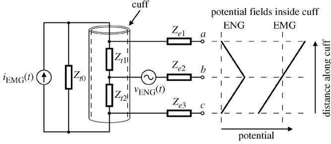
Fig. 1. Lumped-impedance model of the cuff and idealized ENG and EMG potentials inside the cuff [6], [12]. Typical impedance values:  $Z_{t0} = 200 \Omega$ ,  $Z_{t1,2} = 1.25 \text{ k}\Omega$ ,  $Z_{e1,2,3} = 1 \text{ k}\Omega$ .
