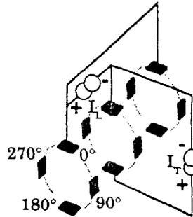
Fig. 1: Geometry of the multiple contact nerve cuff electrode.  $I_L$  is the longitudinal stimulus current, and  $I_T$  is the transverse field steering current. Each of the four tripoles was connected as shown.
