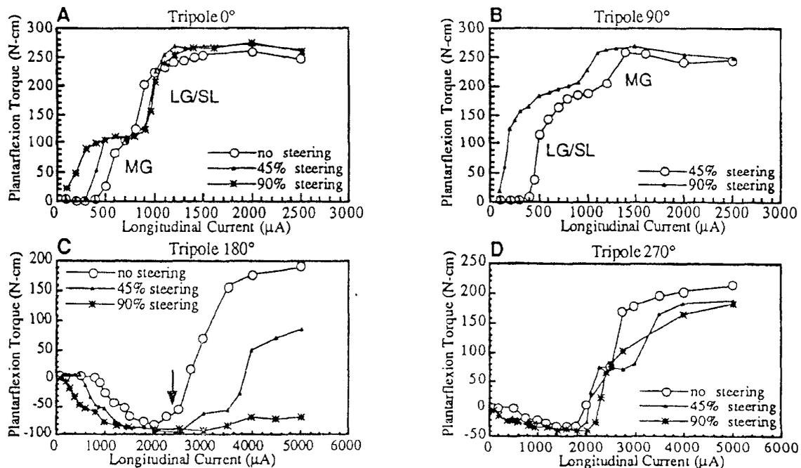
Figure 2: Ankle joint torque as a function of longitudinal stimulus current with different transverse steering current magnitudes.
