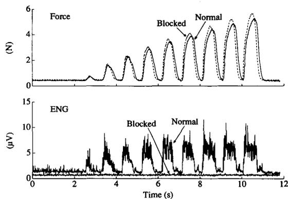
Fig. 3. Validation of the artifact removal method. Solid traces show the force applied on the footpad (top) and the normal sampled ENG (bottom) during quasi-sinusoidal stimulation of the four plantarflexor muscles. The dashed traces show a similar trial, after sensory nerve conduction between the foot and the recording cuff was blocked. Further description in text.
