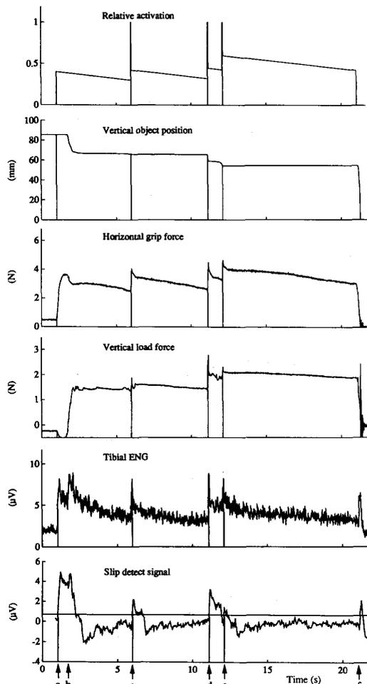
Fig. 6. Slip detection during an increase in external load, with subsequent compensation. Initial part of the run was as in Fig. 5, but as soon as a slip was detected by the controller (dotted line) a doublet pulse was elicited and the pulse width of subsequent stimuli was increased by 40%, which stopped the fall and held the object securely afterward. The RBI-ENG (dotted trace) is shown as it was sampled, and the solid trace is the RBI-ENG low pass filtered at 5 Hz. Data from cat 10.
