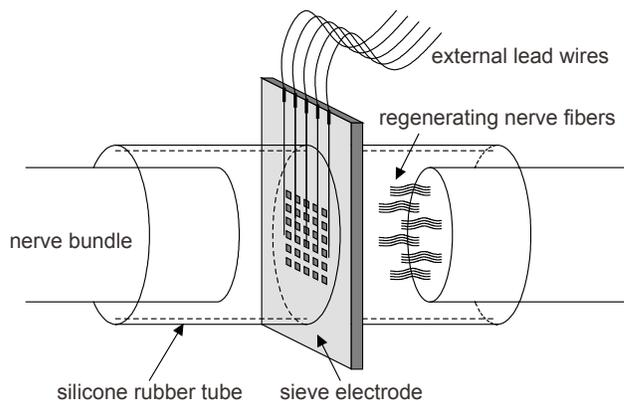
Fig. 1. Schematic diagram of the sieve electrode.
