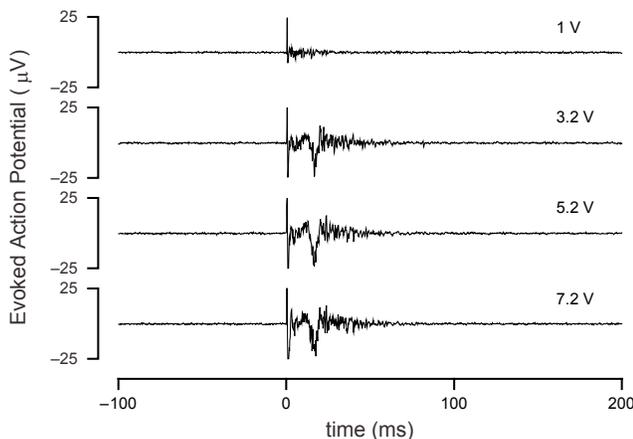
Fig. 5. Evoked action potential recorded from the sieve electrode.
