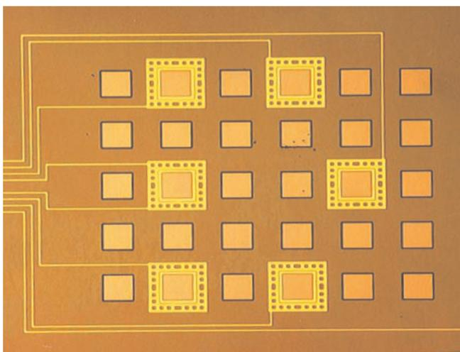
Fig. 2. Design of the diaphragm of the sieve electrode. The photograph shows the diaphragm with 30 penetrating square holes (100  $\mu\text{m}$  in one side). Six of the 30 holes were rimmed with the Au rings.
