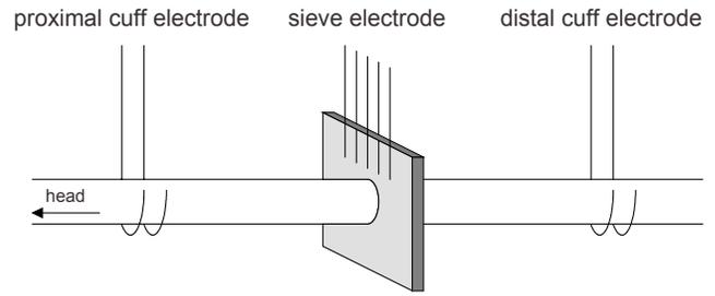
Fig. 3. Configuration of cuff electrodes and sieve electrode to examine evoked action potential.
