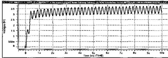
Figure 7. The simulating result of voltage rectifier circuit.
