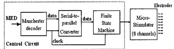
Figure 5. Functional blocks of the control circuit.
