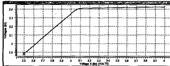
Figure 9. The output of voltage regulator versus the supply voltage.
