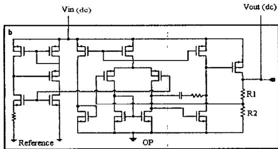
Figure 4. Circuit implementation of voltage regulator.
