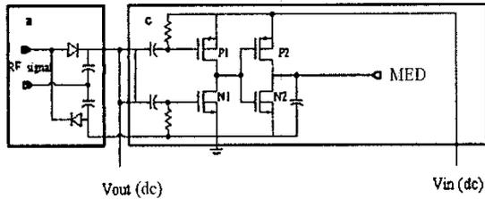
Figure 2. Circuit implementation of voltage rectifier and demodulator.
