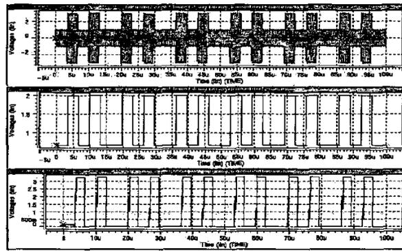
Figure 10. The simulation results of the demodulator.
