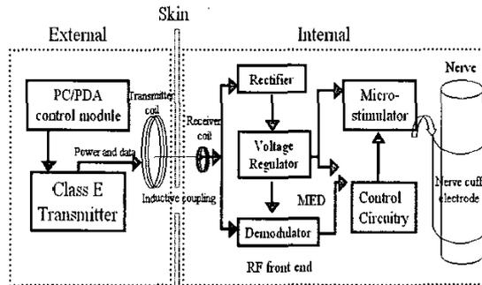
Figure 1. Block diagram of a micro-stimulator system.
