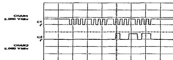
Figure 11. Output waveform of Manchester decoder.
