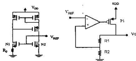
Figure 3. Architecture of voltage reference and voltage regulator.
