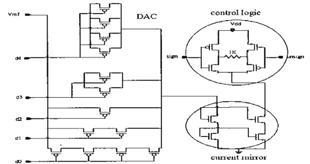
Figure 6. Circuit diagram of constant current source.
