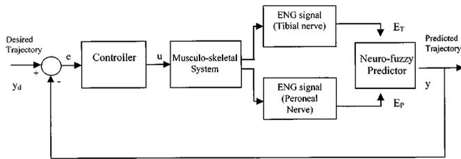
Fig. 1. Diagram of the implementing system for standing control using natural sensory information. The information extracted from the ENG signals recorded from muscle afferents will be used to modify the stimulation parameters in a closed-loop paradigm.
