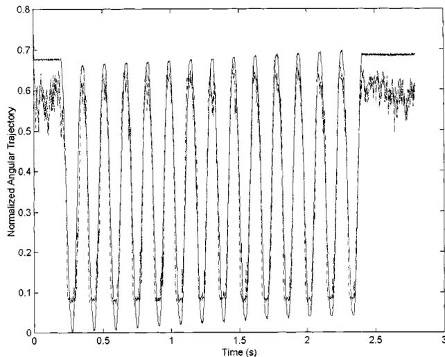
Fig. 10. The predicted ankle profile (dash-dotted line) and the actual one (solid line) for the test set of trajectory #7 (Rabbit #3).
