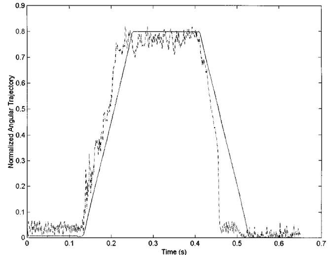
Fig. 9. The predicted ankle profile (dash-dotted line) and the actual one (solid line) for the test set of trajectory #6 (Rabbit #3).
