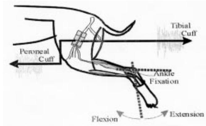
Fig. 2. Schematic illustration of the implantation sites. The cuff electrodes were used to record the ENG signals from the tibial and peroneal nerve while the ankle joint of the Rabbits was rotated by using a servo-motor.
