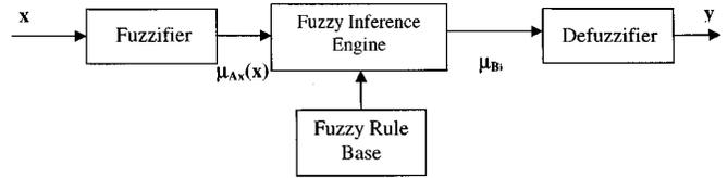
Fig. 5. Diagram of a FS. A FS is composed by four subsystems: 1) the fuzzifier which transforms real data into subjective fuzzy values; the fuzzy rule base which represents the core of the FS incorporating the knowledge used (in this application) to extract the angular information; the inference engine which is used to infer the fuzzy rules with respect to the fuzzified data; and the defuzzifier which transforms fuzzy variables into real data.
