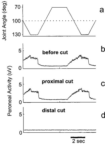
Fig. 4. Experiments to verify the afferent origin of the ENG signals recorded. Trace (a) indicates the profile imposed to the rabbit ankle. Trace (b) indicates the peroneal nerve recorded activity before any transection. Trace (c) indicates the peroneal nerve recorded activity after a transection proximal to the cuff. Trace (d) indicates the peroneal nerve recorded activity after a transection distal to the cuff. (Reproduced with permission from R. Riso *et al.*[14].)
