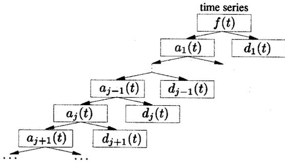
Fig. 4. The hierarchical structure of the MRA generated by wavelets.  $f(t)$  is time series data,  $a_j(t)$  is discrete approximation of  $f(t)$ , and  $d_j(t)$  is discrete detail signal at scale  $j$ .
