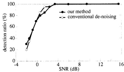
Fig. 6. The detection ratio against various SNR. The frequency components of the neural signal are from 100 Hz to 2 kHz, and those of the noise process are limited with low-pass filter whose cutoff frequency is 4 kHz. The detection ratio of our method is almost same as that of conventional de-noising approach.
