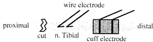
Fig. 2. The arrangement of recording electrodes. A neural signal related to the angle changes of the MTP were recorded from both inside and outside of the tibial nerve with the cuff and the wire electrodes, respectively. The nerve was cut at the proximal side in order to block spinal reflexes.
