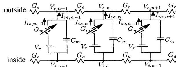
Fig. 1. Electrical circuit representation of a myelinated nerve fiber. The membrane capacitance  $C_m$ , the resting potential  $V_r$ , and the nonlinear membrane conductance  $G_m$  represent the gating of the ionic channels and decide the value of the ionic current  $I_{i_o,n}$  at node  $n$ .  $V_{i,n}$  and  $V_{e,n}$  are the internal and the external potentials,  $G_a$  and  $G_e$  are the axoplasmic and the extracellular conductance, and  $I_{m,n}$  is the membrane current at node  $n$ .
