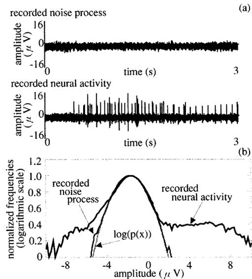
Fig. 3. The recorded time series and their amplitude histogram. (a) The neural activity related to the angle changes of MTP were recorded with wire electrode. (b) The amplitude histograms of the recorded noise process and the recorded neural activity, and  $y = \log(p(x))$  are plotted. Where  $p(x)$  is the probability density function of the normal distribution.
