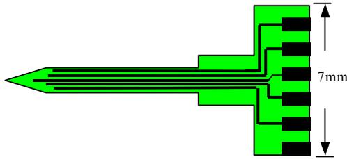
Fig. 1. Schematic diagram of the BCB based neural implant
