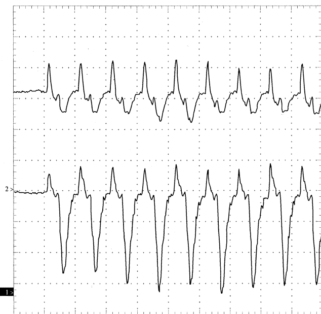
Fig. 14. Recordings of torque. Stimulation was delivered by pulses at 10 pps through two different tripoles of the cuff electrode, producing alternating excitation of the tibial fascicle and plantarflexion (positive torque) and of the peroneal fascicle and dorsiflexion (negative torque). Two recordings from the same preparation are shown; the stimulus amplitude delivered to the tripole inducing plantarflexion was maintained constant, while the stimulus amplitude to the tripole causing dorsiflexion was changed from low level (top recording) to a higher level (bottom recording). Vertical scale: 2.5 N·mm/square. Horizontal scale: 100 ms/square.
