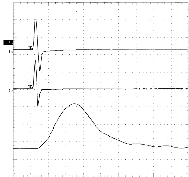
Fig. 12. Simultaneous recordings of CMAP from (top channel) gastrocnemius muscle, (middle) tibialis anterior muscle, and (bottom) ankle torque. Stimulation was delivered by a single pulse through the cuff electrode. The stronger output of the plantarflexor muscles resulted in net plantarflexion (positive torque) despite coactivation of the two muscle groups. Vertical scale: 20 mV/square for CMAPs and 12.5 N·mm/square for torque. Horizontal scale: 10 ms/square.
