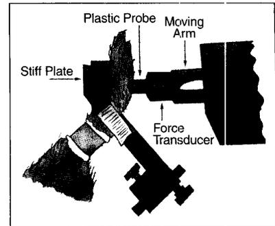
3. The mechanical part of the experimental setup. The rabbit's lower leg is placed in a holder; the foot-pad is indented with a probe instrumented with a force transducer and mounted on the arm of a linear motor.
