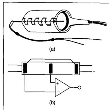
1. (a) The silicone cuff electrode as described in the text (courtesy Dr. M.K. Haugland); the cuff's closure mechanism was developed by Kallesøe, et al. [29]. (b) Tripolar configuration with short-circuited end-contacts.
