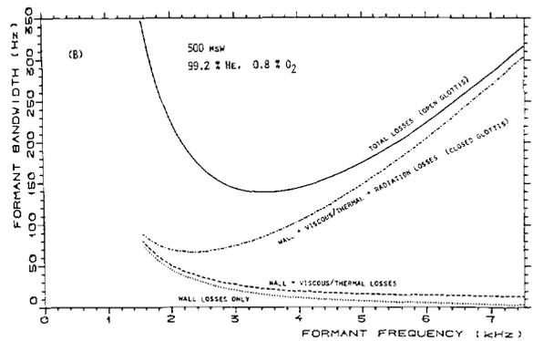
Fig. 2 Relative contributions to formant bandwidth  $B_n$  from the 5 energy loss terms, for (a) air/1 ATA, (b) heliox/48.4 ATA
