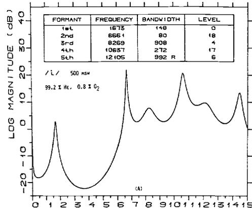
Fig. 4 Vocal tract transfer function  $V(f)$  for the vowel /i/ and nasal /m/ simulated for heliox gas and a pressure of 48.4 ATA
