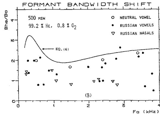
Fig. 5 Ratio of formant frequencies (a) and bandwidths (b) in heliox at 48.4 ATA to air at 1 ATA as function of  $F_0$ . Curves are uniform tube model predictions, markers are multitube model simulations
