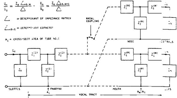
Fig. 3 Transmission-line analog of the multitube vocal tract model (after Flanagan [3])
