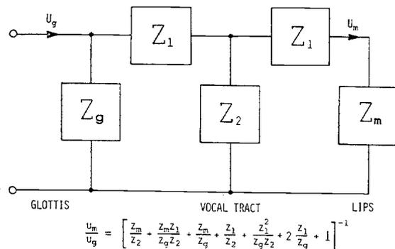
Fig. 1 Transmission-line analog of the uniform single-tube vocal tract model
