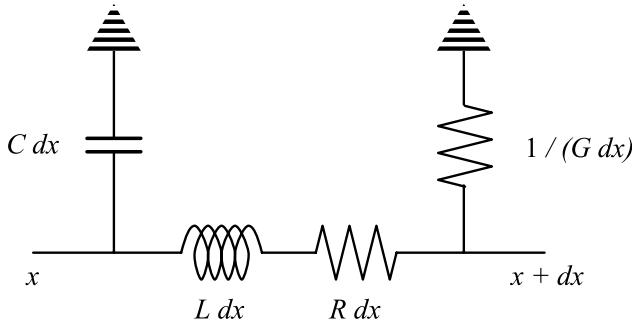
**Fig. 2** Schematic of a telegraph wire
