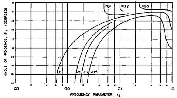
FIG. 6. Low-frequency contours of normalized shell reactance for  $m = 1, \nu = \frac{1}{3}, h/a = 10^{-2}$ .
