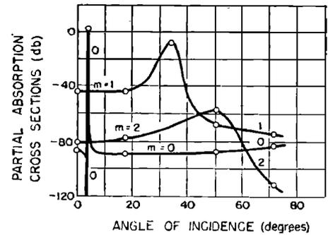
FIG. 9. Partial absorption coefficients of shell as function of angle of incidence  $\theta$  assuming as inside termination an ingoing wave. Results computed for a low frequency ( $x_L=0.02$ ) for a shell with  $\nu=\frac{1}{3}$ ,  $h/a=10^{-2}$ .
