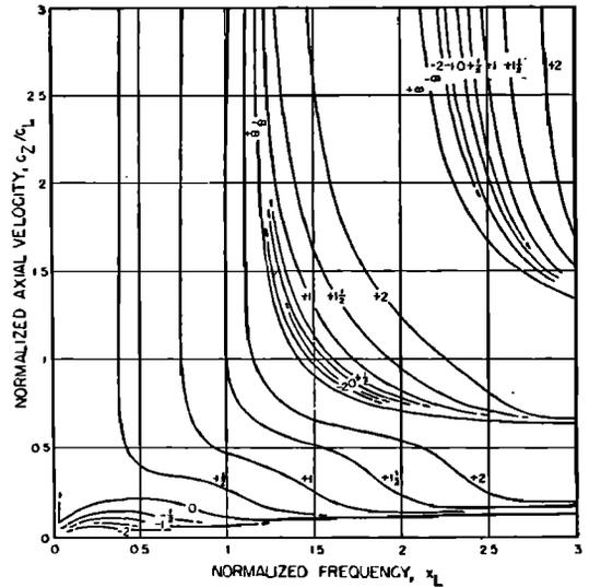
FIG. 4. Contours of normalized shell reactance for  $m=2$ ,  $\nu=\frac{1}{3}$ ,  $h/a=10^{-2}$ .
