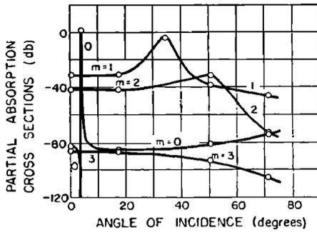
FIG. 8. Partial absorption coefficients of shell as function of angle of incidence  $\theta$  assuming a  $\rho c$  normal impedance inside. Results computed for a low frequency ( $x_L=0.02$ ) for a shell with  $\nu=\frac{1}{3}$ ,  $h/a=10^{-2}$ .
