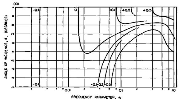
FIG. 7. Low-frequency contours of normalized shell reactance for  $m = 2, \nu = \frac{1}{3}, h/a = 10^{-2}$ .
