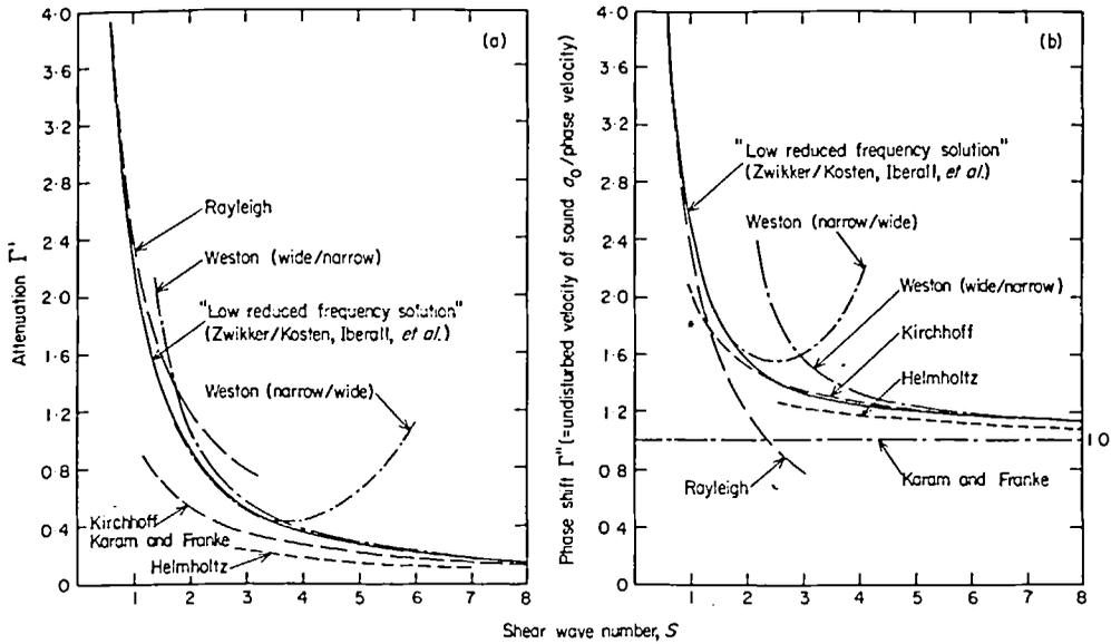
Figure 2. (a) Attenuation  $\Gamma'$  and (b) phase shift  $\Gamma''$  as functions of shear wave number.
