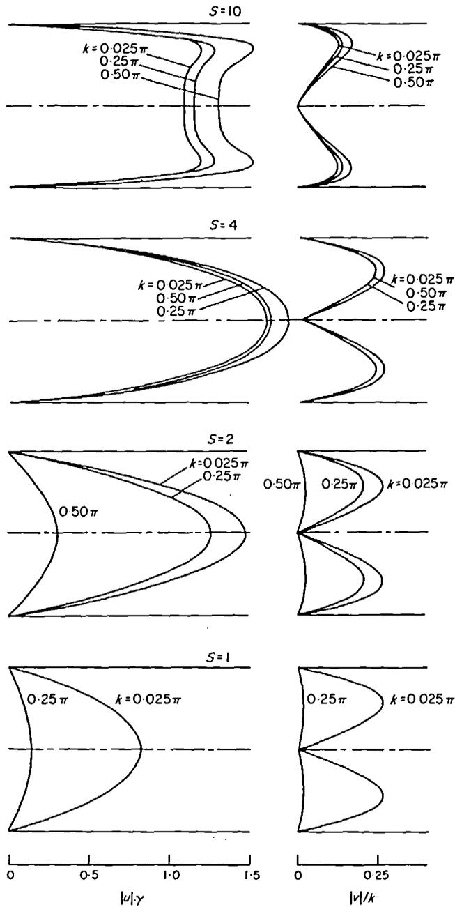
Figure 11. Velocity distributions in radial and axial directions.
