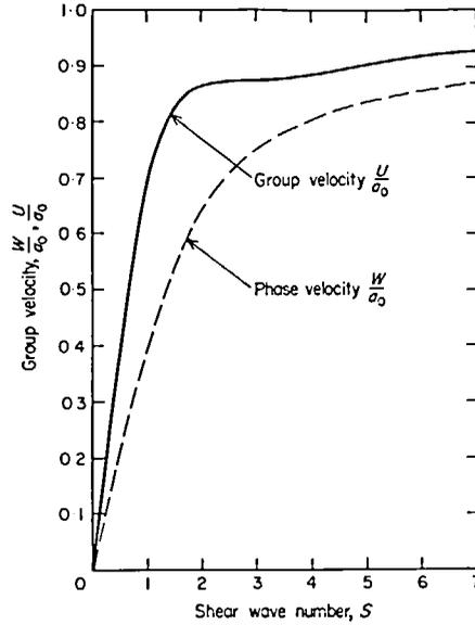
Figure 7. Phase velocity and group velocity according to the “low reduced frequency solution”.
