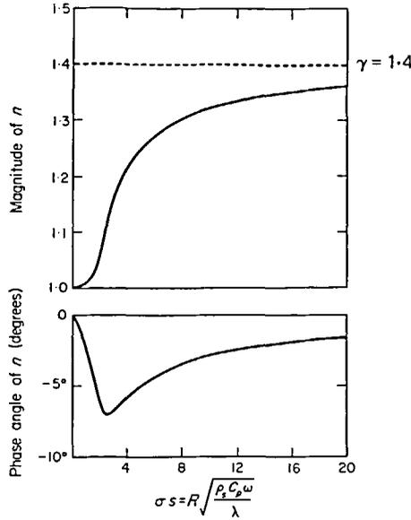
Figure 4. "Polytropic constant",  $n$ , as a function of  $\sigma s$ .
