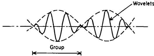
Figure 6. Sketch of a modulated wave showing group and wavelet components.
