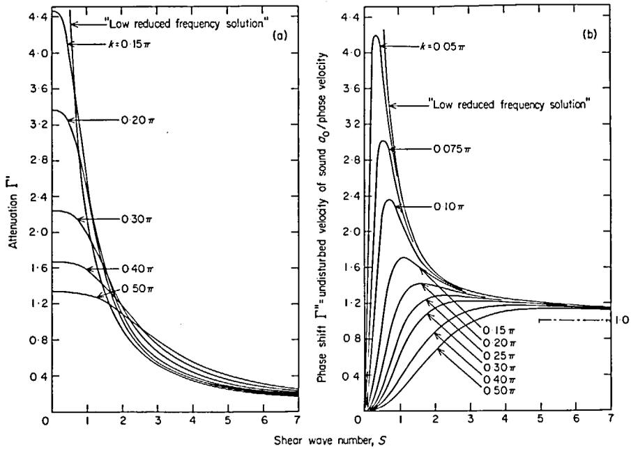
Figure 9. Exact solution of (a)  $\Gamma'$  and (b)  $\Gamma''$  as functions of shear wave number and reduced frequency.
