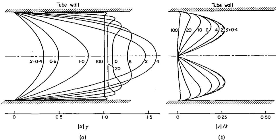
Figure 5. Velocity distribution in (a) axial direction and (b) radial direction according to the "low reduced frequency solution".
