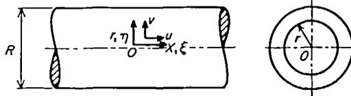
Figure 1. Co-ordinate system. Dimensionless co-ordinates:  $\xi = \omega x/a_0$ ;  $\eta = r/R$ .
