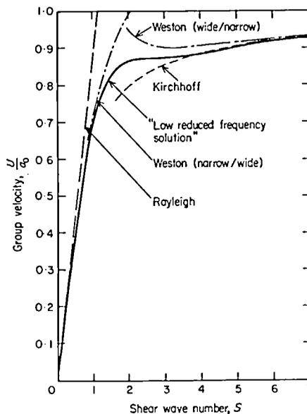
Figure 8. Comparison of various solutions for the group velocity.
