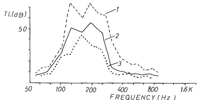
Fig. 10 Effect of the free cross section of the duct on the transmission loss
