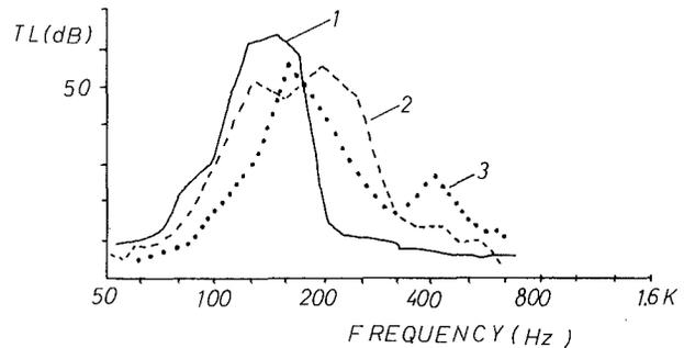
Fig. 9 Effect of the length of the openings of the resonators on the transmission loss
