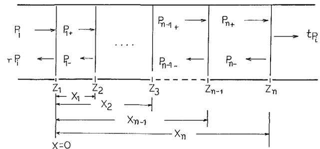
Fig. 4 One-dimensional idealized model of duct
