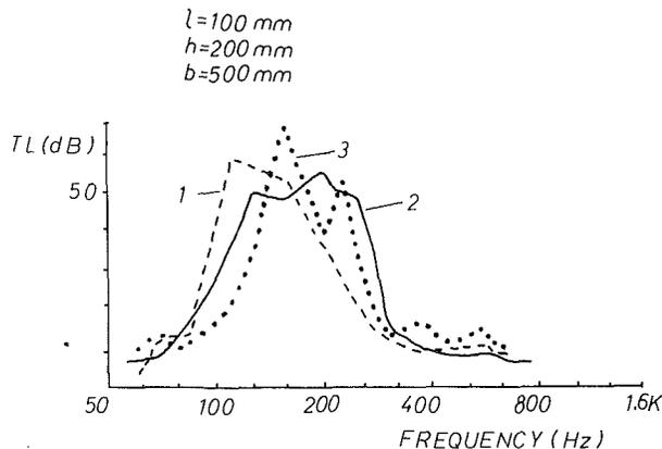
Fig. 8 Effect of the ordering of the resonators on the transmission loss
