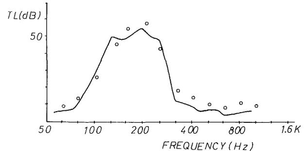
Fig. 7 Transmission loss of a duct with eight resonators of different length. Predicted —, measured  $\circ$ .
