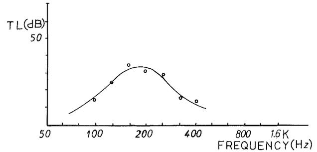
Fig. 6 Transmission loss of a duct with four identical resonators. Predicted —, measured  $\circ$ .
