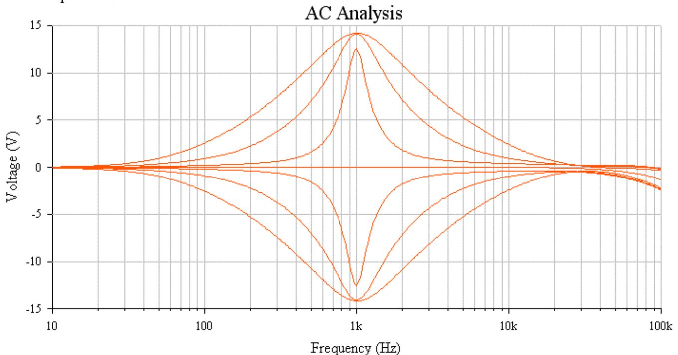
**Fig. 7: Effect Of Q On Bandwidth In A Graphic Equalizer**
