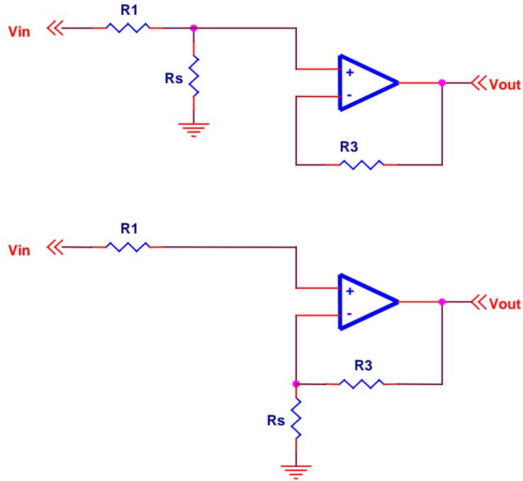
**Fig. 5: Gain Circuit at Either End of Potentiometer Travel**
