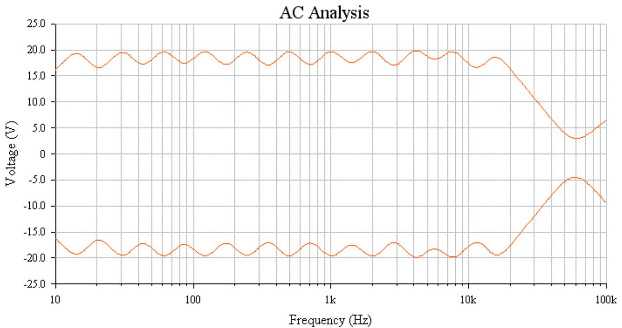
**Fig. 10: Frequency Response Of A 1-Octave Equalizer**
