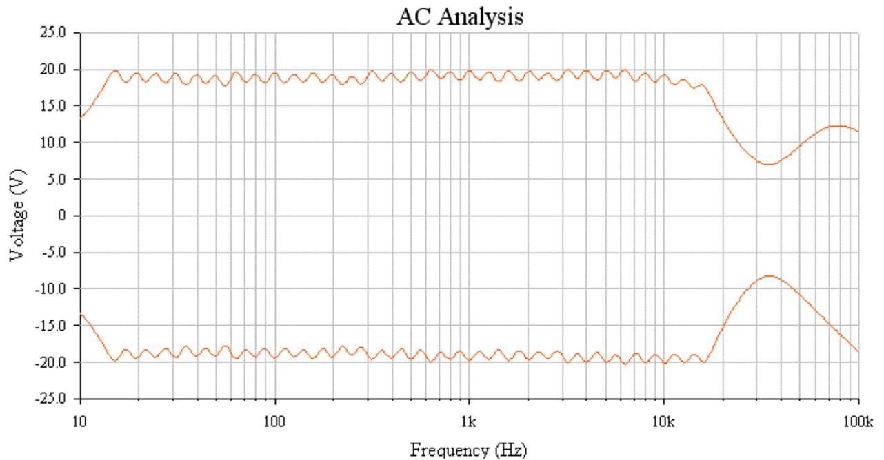
**Fig. 11: Frequency Response Of A  $\frac{1}{3}$ -Octave Equalizer**
