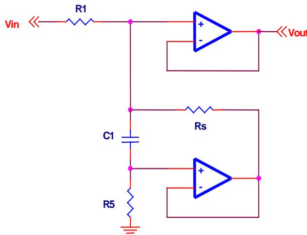
**Fig. 2: High-Pass Filter Using A Simulated Inductor**
