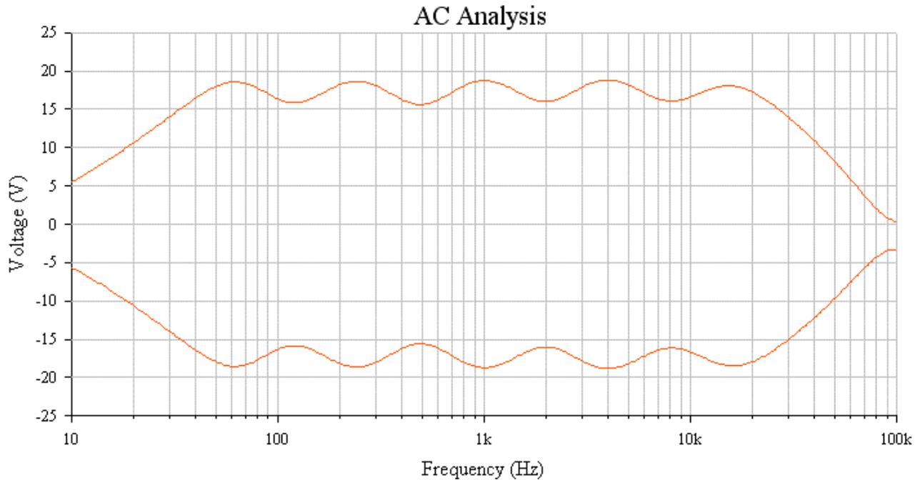
**Fig. 8: Frequency Response Of A 2-Octave Equalizer**
