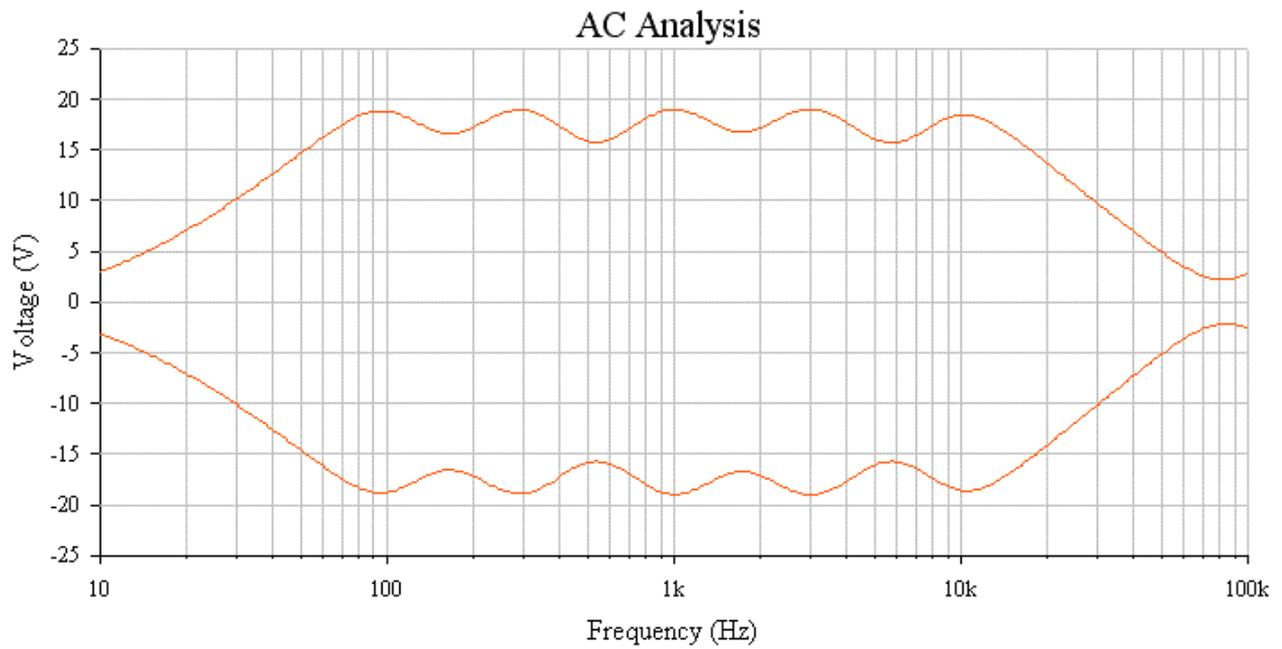
**Fig. 9: Frequency Response Of A Pseudo 2 Octave Equalizer**
