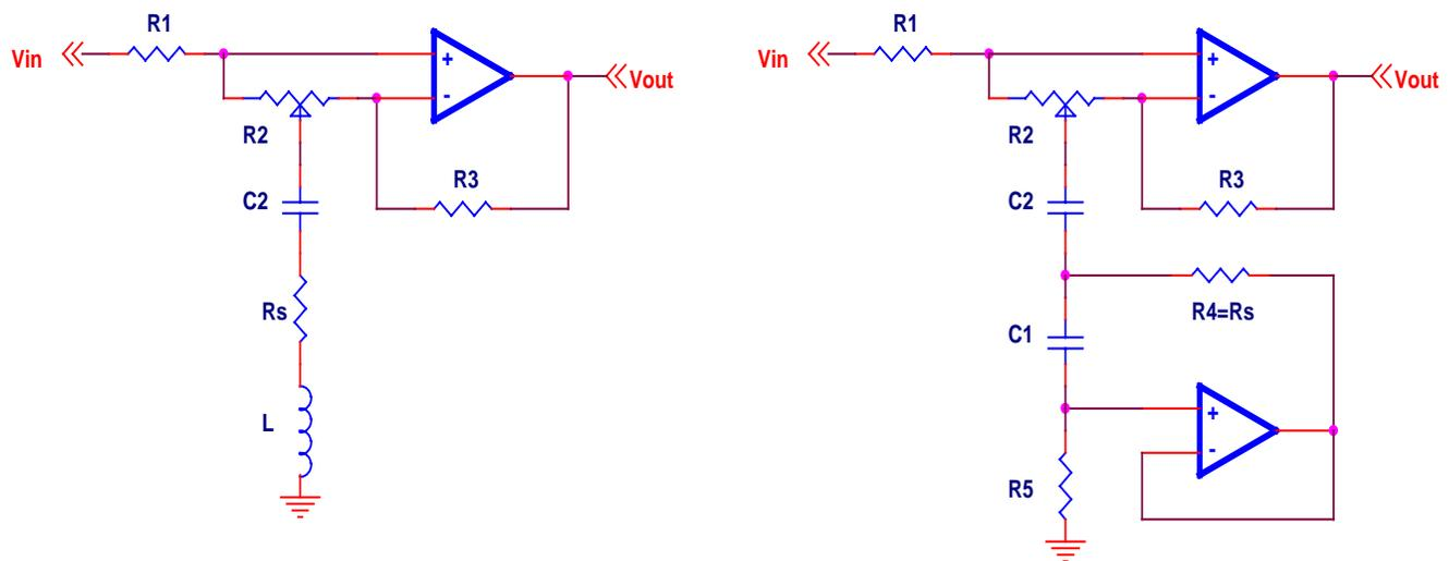
**Fig. 4: Graphic Equalizer (Physical Inductor On Left, Simulated Inductor On Right)**
