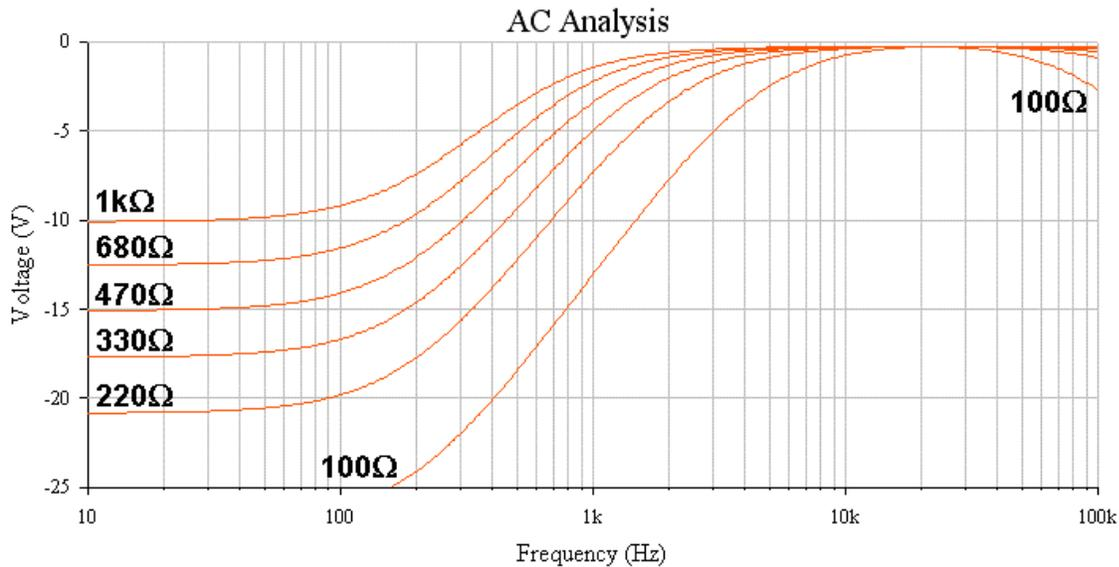
**Fig. 3: Response Of Simulated Inductor High-Pass Filter**
