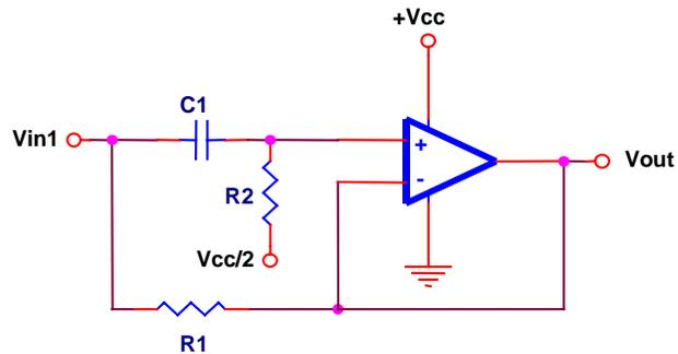
**Fig. 1: A Simulated Inductor Circuit**
