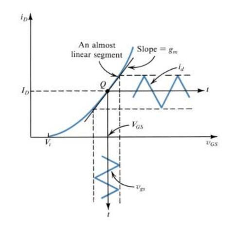
Small-signal operation of the enhancement MOSFET amplifier.
