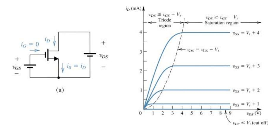
(a) An n-channel enhancement-type MOSFET with  $v_{GS}$  and  $v_{DS}$  applied and with the normal directions of current flow indicated. (b) The  $i_D - v_{DS}$  characteristics for a device with  $V_t = 1$  V and  $k'_n(W/L) = 0.5$  mA/V<sup>2</sup>.
