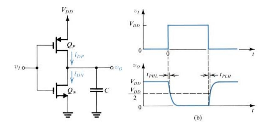
Dynamic operation of a capacitively loaded CMOS inverter: (a) circuit; (b) input and output waveforms.
