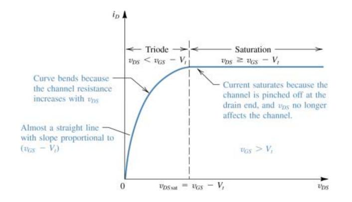
The drain current  $i_D$  versus the drain-to-source voltage  $v_{DS}$  for an enhancement-type NMOS transistor operated with  $v_{GS} > V_t$ .
