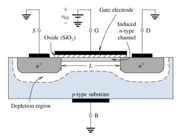
The enhancement-type NMOS transistor with a positive voltage applied to the gate. An n channel is induced at the top of the substrate beneath the gate.
