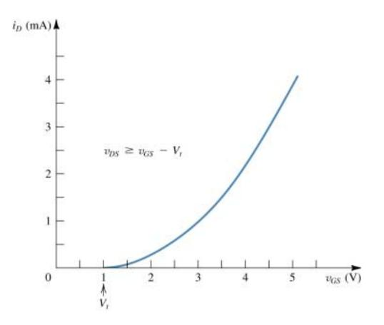
The  $i_D$  -  $v_{GS}$  characteristic for an enhancement-type NMOS transistor in saturation  $(V_t = 1 \text{ V and } k'_n(W/L) = 0.5 \text{ mA/V}^2).$
