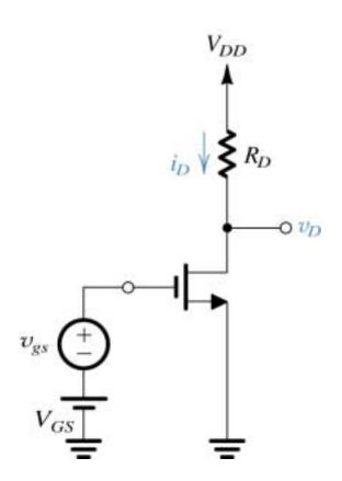
Conceptual circuit utilized to study the operation of the MOSFET as an amplifier.
