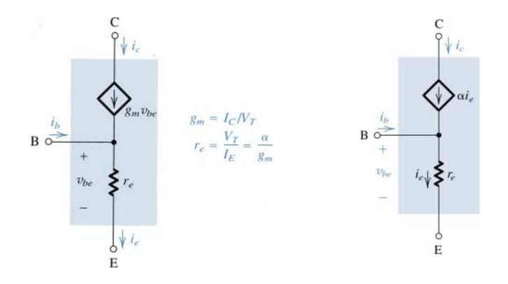
Two slightly different versions of what is known as the *T model* of the BJT. The circuit in (a) is a voltage-controlled current source representation and that in (b) is a current-controlled current source representation. These models explicitly show the emitter resistance  $r_e$  rather than the base resistance  $r_{\Pi}$  featured in the hybrid- $\pi$  model.
