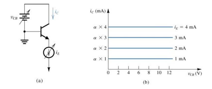
The  $i_C - v_{CB}$  characteristics for an npn transistor in the active mode.
