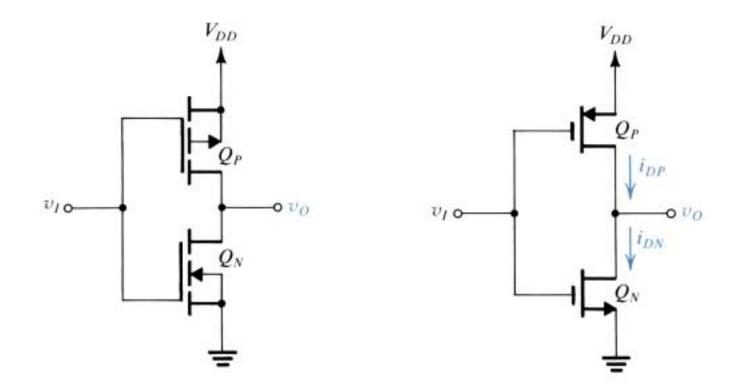
(a) The CMOS inverter. (b) Simplified circuit schematic for the inverter.
