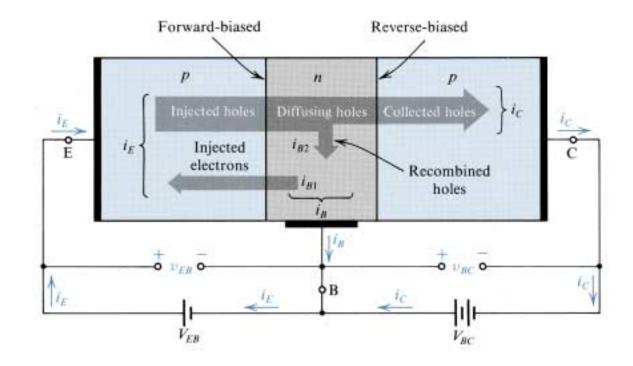
Current flow in an pnp transistor biased to operate in the active mode.
