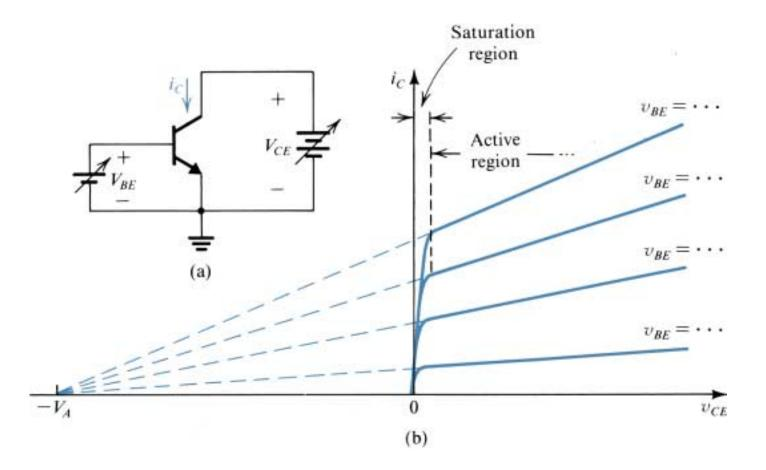
(a) Conceptual circuit for measuring the  $i_C v_{CE}$  characteristics of the BJT. (b) The  $i_C v_{CE}$  characteristics of a practical BJT.
