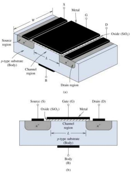
Physical structure of the enhancement-type NMOS transistor: (a) perspective view; (b) cross section. Typically L = 1 to 10 µm, W = 2 to 500 µm, and the thickness of the oxide layer is in the range of 0.02 to 0.1 µm.
