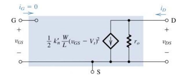
Large-signal equivalent circuit model of the *n*-channel MOSFET in saturation, incorporating the output resistance  $r_o$ . The output resistance models the linear dependence of  $i_D$  on  $v_{DS}$  and is given by  $r_o \cong V_A I_D$ .
