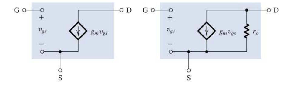
Small-signal models for the MOSFET: (a) neglecting the dependence of  $i_D$  on  $v_{DS}$  in saturation (channel-length modulation effect); and (b) including the effect of channel-length modulation modeled by output resistance  $r_o = |V_A/I_D$ .
