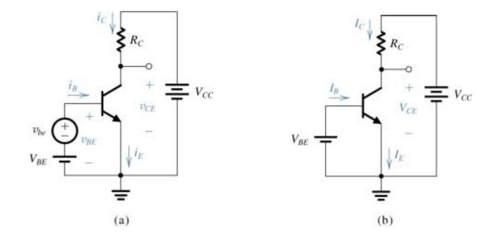
(a) Conceptual circuit to illustrate the operation of the transistor of an amplifier. (b) The circuit of (a) with the signal source  $v_{be}$  eliminated for dc (bias) analysis.
