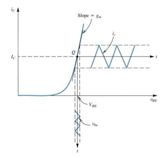
Linear operation of the transistor under the small-signal condition: A small signal  $v_{be}$  with a triangular waveform is superimpose din the dc voltage  $V_{BE}$ . It gives rise to a collector signal current  $i_c$ , also of triangular waveform, superimposed on the dc current  $I_C$ .  $I_c = g_m v_{be}$ , where  $g_m$  is the slope of the  $i_c - v_{BE}$  curve at the bias point Q.
