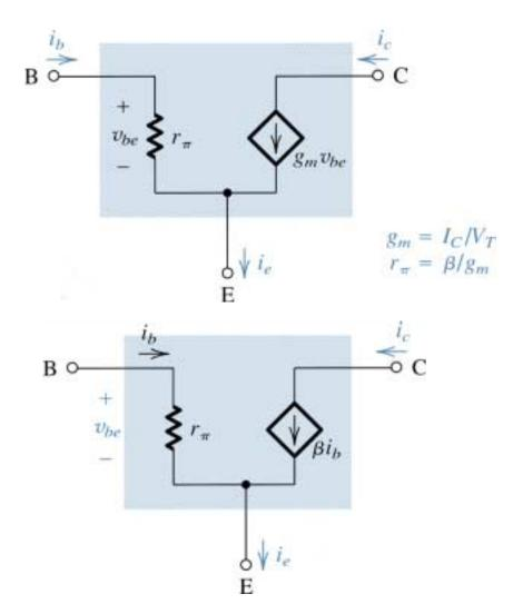
Two slightly different versions of the simplified hybrid- $\Pi$  model for the small-signal operation of the BJT. The equivalent circuit in (a) represents the BJT as a voltage-controlled current source (a transconductance amplifier) and that in (b) represents the BJT as a current-controlled current source (a current amplifier).
