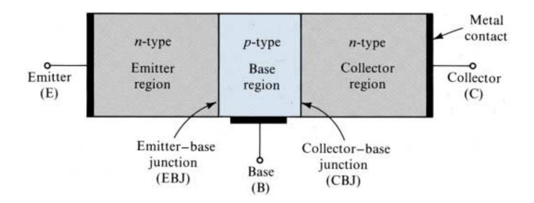
A simplified structure of the *npn* transistor.
