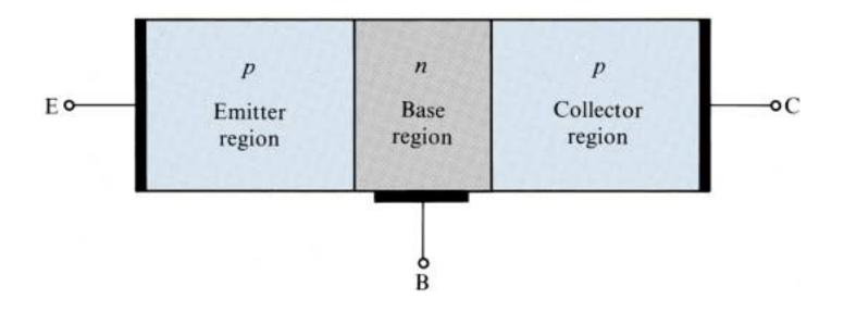
A simplified structure of the *pnp* transistor.
