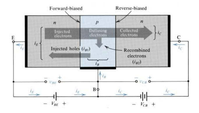
Current flow in an *npn* transistor biased to operate in the active mode, (Reverse current components due to drift of thermally generated minority carriers are not shown.)
