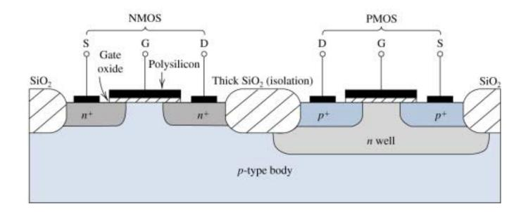
Cross section of a CMOS integrated circuit. Note that the PMOS transistor is formed in a separate n-type region, known as an n well. Another arrangement is also possible in which an n-type body is used and the n device is formed in a p well.
