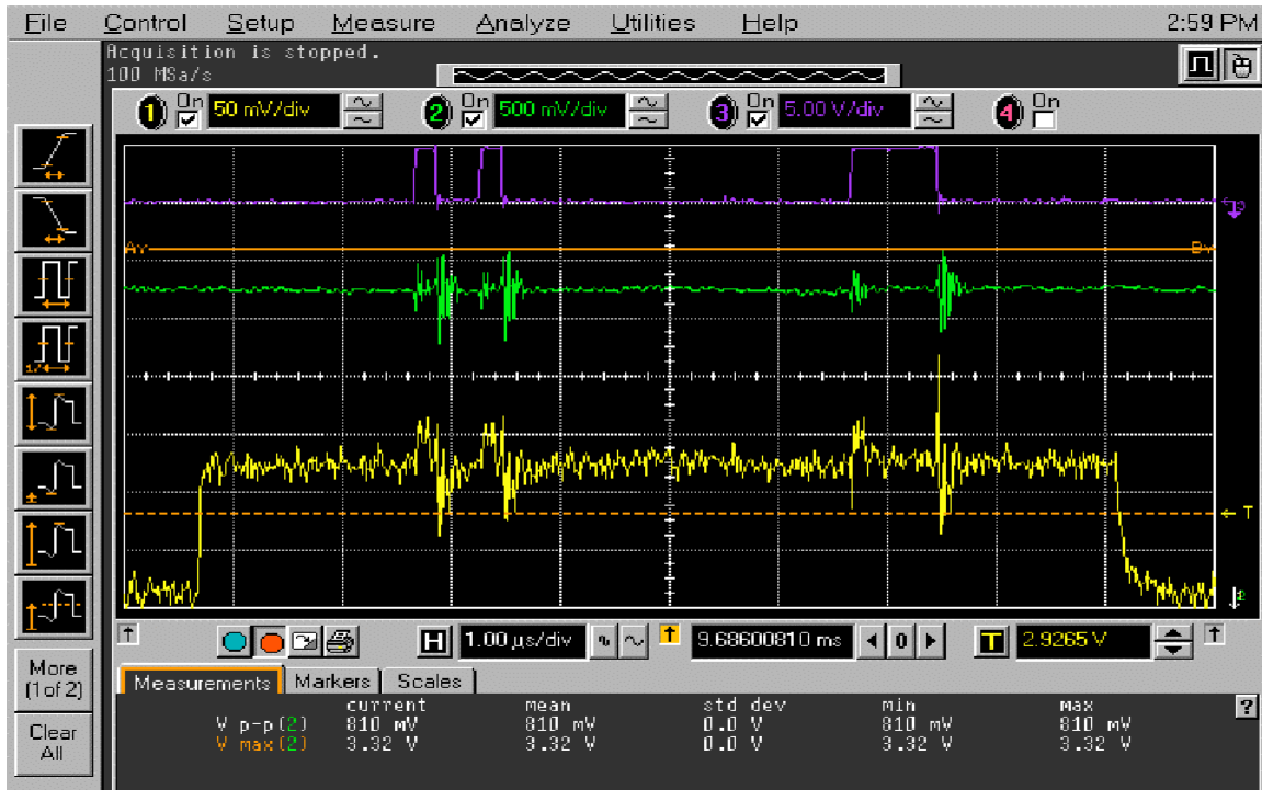
Fig. 4: In this scope photo, the upper trace was taken at JP1 (digital word to the digital potentiometers), the middle trace on JP5 (noise on the adjacent analog trace) and the lower yellow trace is at TP10 (noise at the output of the 16-bit DAC)
