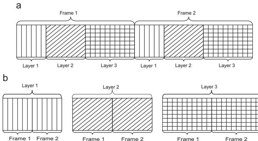
Fig. 2. Layered video storage structure.
