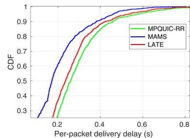
Fig. 16. Per-packet delivery delay distribution when a video client requests the video data as encoded in [52].
