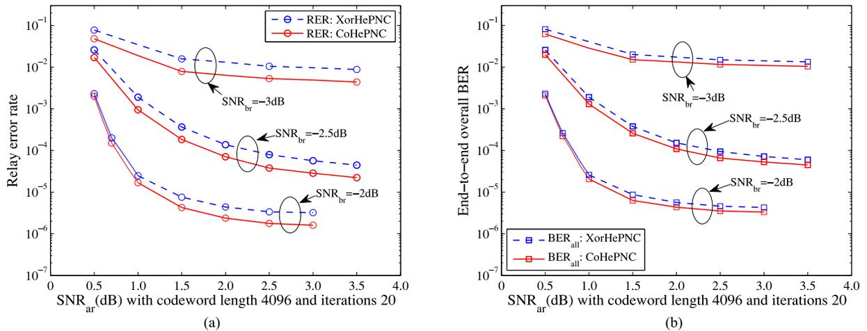
Fig. 7. CoHePNC vs XOR HePNC with iterations = 20, duplicate  $q = 3$  under fast Rayleigh fading channels. (a) Relay error rate. (b) End-to-end BER.
