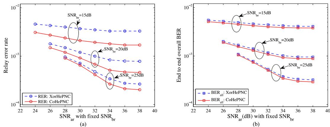
Fig. 9. Block fading channel with codeword length 4096 and iterations 20. (a) Relay error rate. (b) End-to-end BER.
