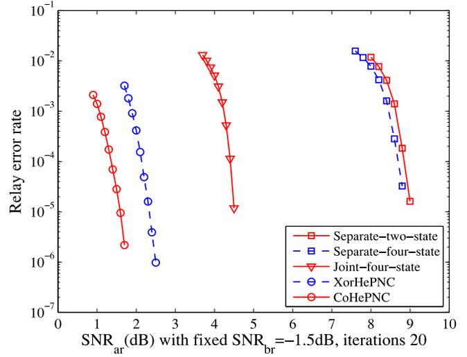
Fig. 5. Comparison of several decoding algorithms.
