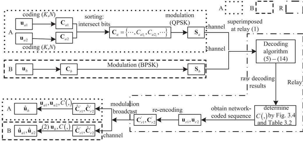
Fig. 1. Procedure diagram of integrating channel coding into HePNC in a link-to-link manner.
