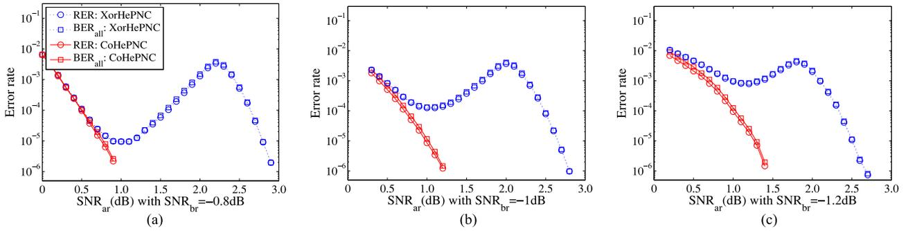
Fig. 6. CoHePNC vs XOR HePNC with codeword length 4096 bits, iterations = 20 and duplicate  $q = 3$  under Gaussian channels. (a)  $\text{SNR}_{br} = -0.8$  dB, (b)  $\text{SNR}_{br} = -1.0$  dB, (c)  $\text{SNR}_{br} = -1.2$  dB.
