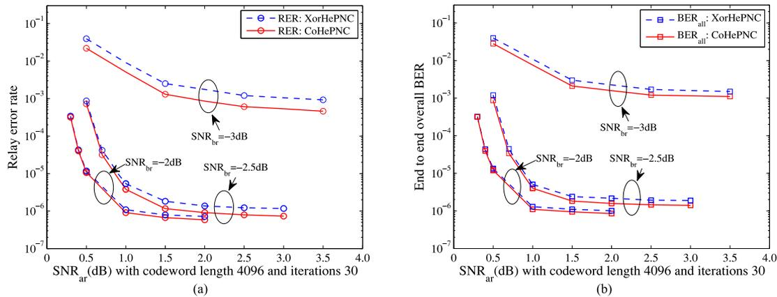
Fig. 8. CoHePNC vs XOR HePNC with iterations = 30, duplicate  $q = 3$  under fast Rayleigh fading channels. (a) Relay error rate. (b) End-to-end BER.
