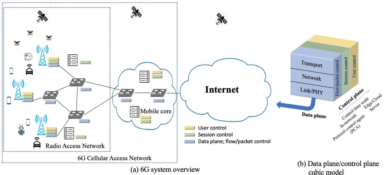
Fig. 3. 6G system overview and data/control-plane protocol model.
