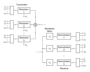
FDM system with two levels of modulation.
