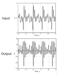
Evidently, differentiation tends to enhance high-frequency components and weaken low-frequency components somewhat like highpass filtering.
