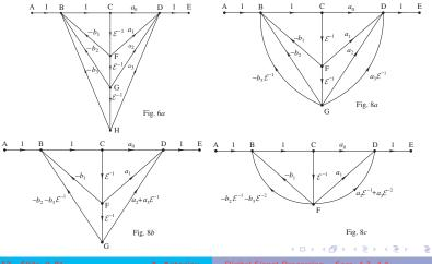
Combine parallel branches in Fig. 8c, eliminate node F in Fig. 8d and node C in Fig. 8e:
