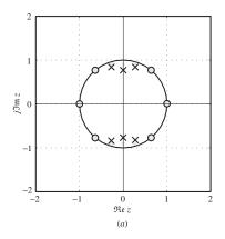
$\begin{aligned} z_1, z_2 &= \pm 1 \quad z_3, z_4 = 0.638 \pm j0.770 \quad z_5, z_6 &= -0.638 \pm j0.770 \\ p_1, p_2 &= \pm j0.902 \quad p_3, p_4 = 0.274 \pm j0.770 \quad p_5, p_6 &= -0.274 \pm j0.770 \end{aligned}$
