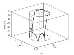
The *intersection* between surface |H(z)| and the cylinder, i.e., the solid curve, is the *amplitude response*.
