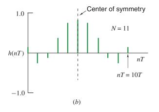
In most applications only the group delay needs to be constant in which case the phase response can have the form
