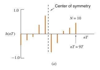
• For *odd* N, the impulse response is antisymmetrical about sample (N-1)/2 as shown:
