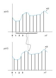
► For the case of a forward- or central-difference formula, the digital filter obtained turns out to be noncausal.
