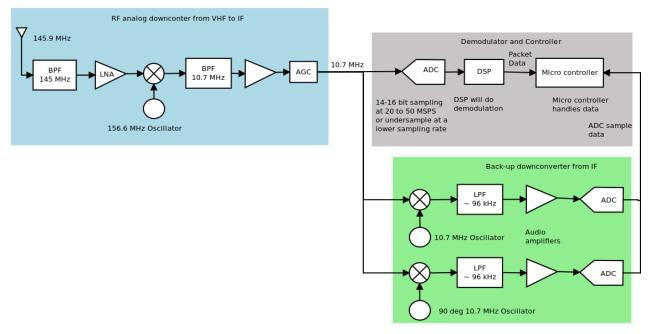
The proposed project is to complete both the up-converter and down-converter RF analog boards shown above in blue in the transmitter and receiver block diagram, respectively. Completion includes finishing the design, building and then testing the boards.
