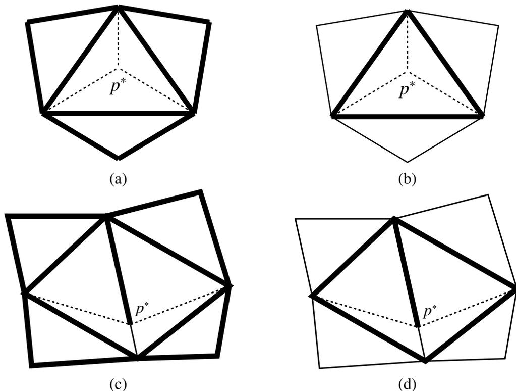
Figure 3.3: Example of determining the newly suspect edges after the insertion of the point  $p^*$  inside a face: (a) first case, (b) second case, and on the edge: (c) first case, (d) second case.
