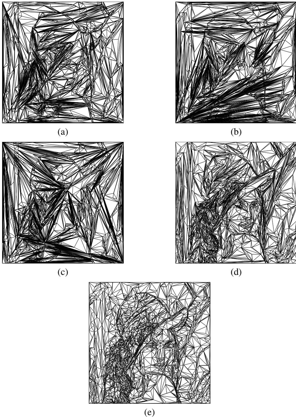
Figure 3.12: The triangulations obtained for the lena image at a sampling density of 1% with the main edge-flip criterion chosen as (a) ABN (28.55 dB), (b) DP (22.75 dB), (c) SE (24.20 dB), (d) DLP (28.22 dB), and (e) JNDSE (29.41 dB), respectively.
