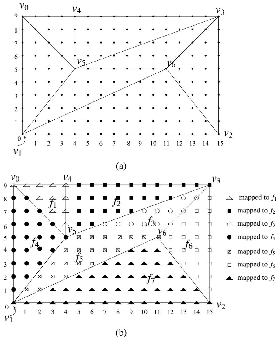
Figure 2.8: An example of how points are assigned to only one face. (a) A triangulation on a rectangular grid, and (b) a triangulation with only vertices and points on edges shown.
