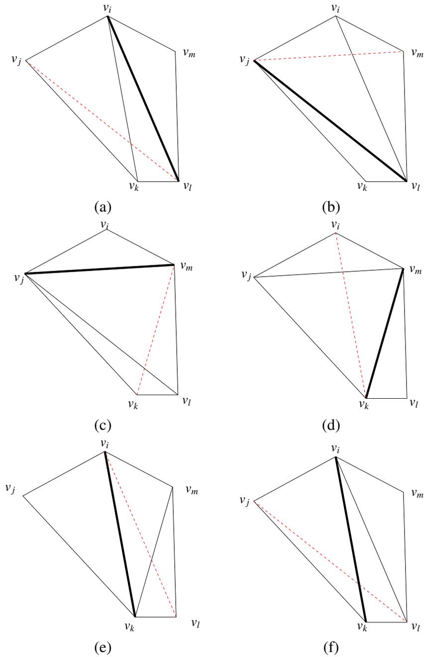
Figure 3.16: An example of cycle in mesh generation. In each triangulation, dashed line denotes the new edge from flipping an old non-optimal edge; dark line denotes the next suspect edge that will be tested for optimality; the regular lines are the edges in the current triangulation.
