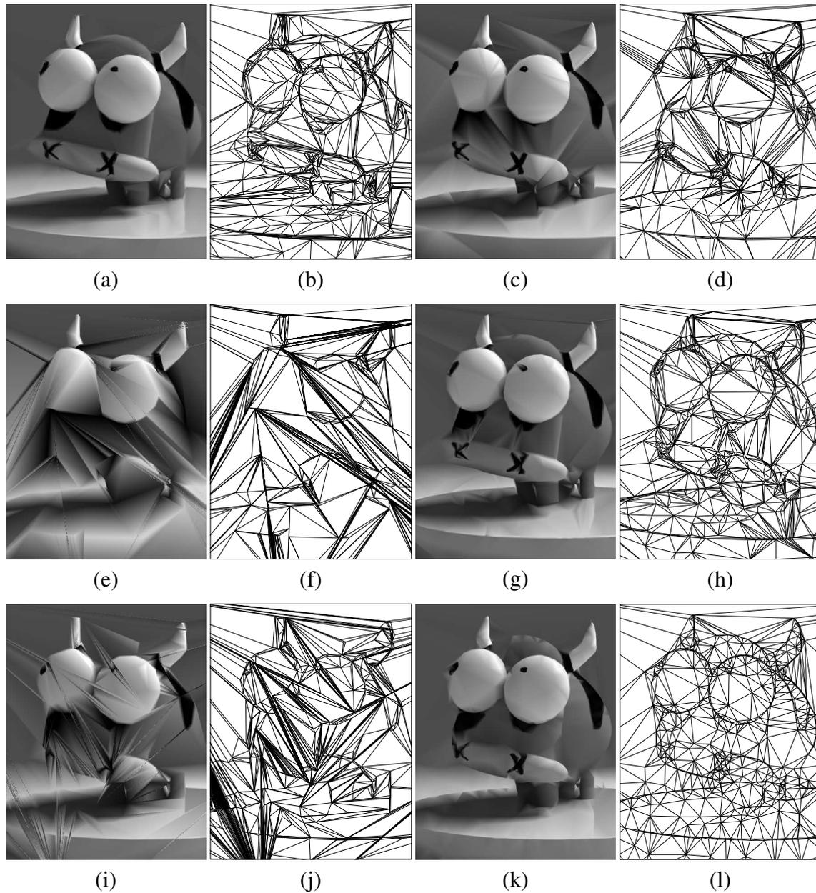
Figure 3.17: Part of the image approximation obtained for the bull image at a sampling density of 0.125% with the (a) proposed (36.48 dB), (c) GH (26.55 dB), (e) R (19.26 dB), (g) GH2 (33.12 dB), (i) R2 (25.83 dB), and (k) AT (33.12 dB), methods and (b), (d), (f), (h), (j), and (l) their corresponding triangulations.
