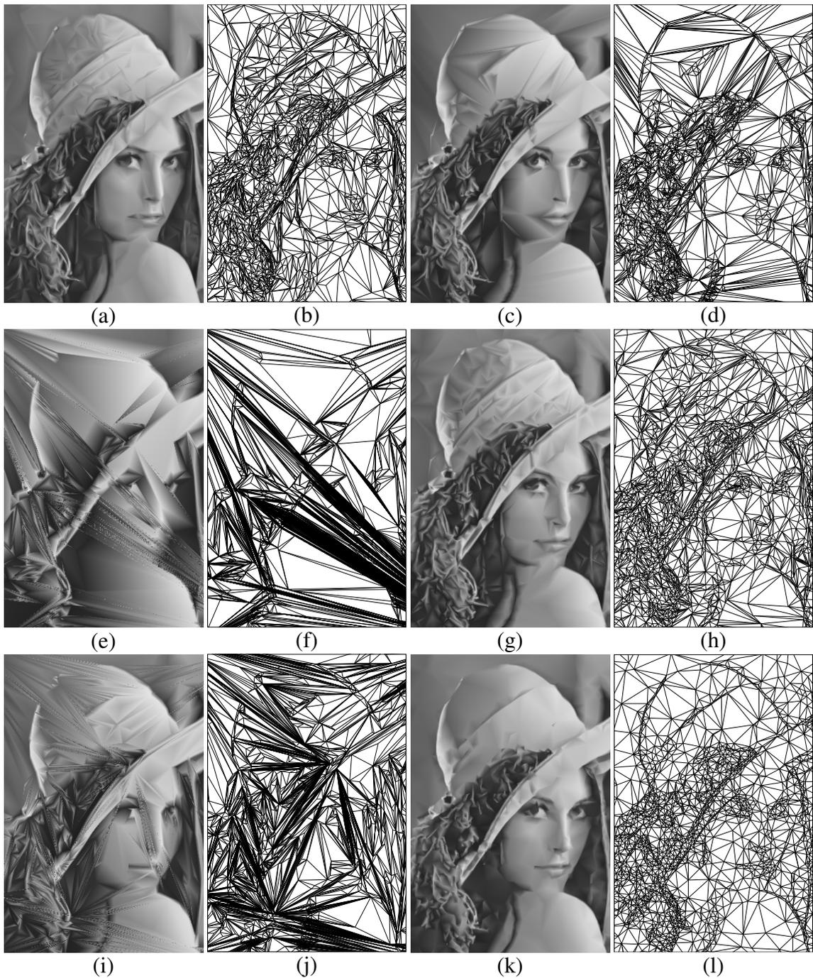
Figure 3.18: Part of the image approximation obtained for the lena image at a sampling density of 1% with the (a) proposed (30.16 dB), (c) GH (25.27 dB), (e) R (19.34 dB), (g) GH2 (28.51 dB), (i) R2 (24.20 dB), and (k) AT (29.12 dB), methods and (b), (d), (f), (h), (j), and (l) their corresponding triangulations.
