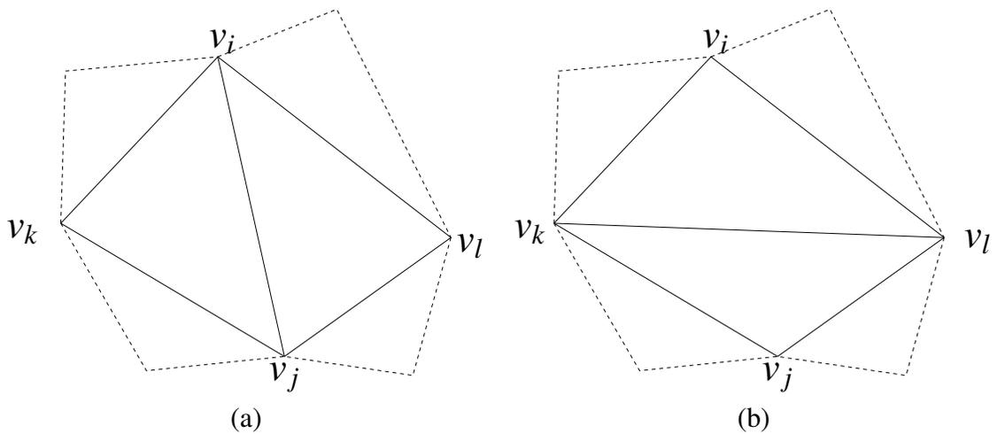
Figure 2.6: Edge flip example. Part of (a) a triangulation with an edge  $\overline{v_i v_j}$  and (b) the new triangulation obtained after the edge  $\overline{v_i v_j}$  is transformed to the edge  $\overline{v_k v_l}$  by an edge flip.
