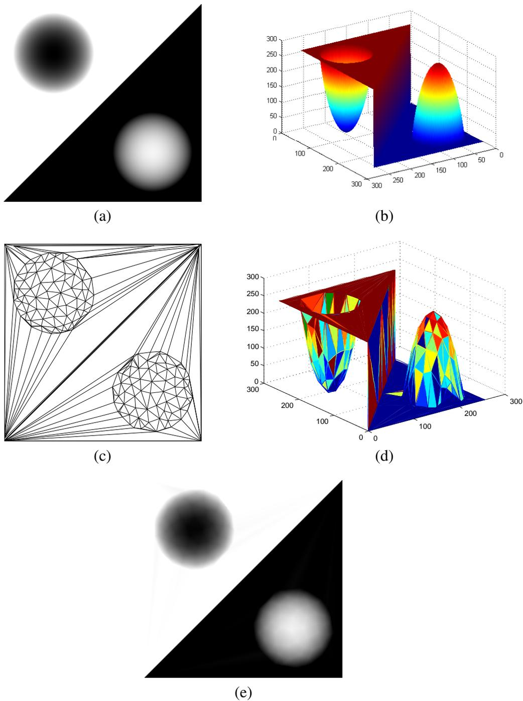
Figure 2.7: Mesh model of an image. (a) Original image, (b) image modelled as surface, (c) triangulation of image domain, (d) resulting triangle mesh , and (e) reconstructed image.
