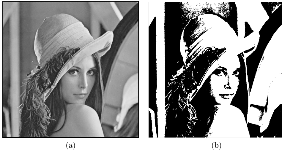
Figure 2.6: An example of image thresholding. The (a) original lena image and (b) the corresponding binary image obtained with \tau = 128 .
