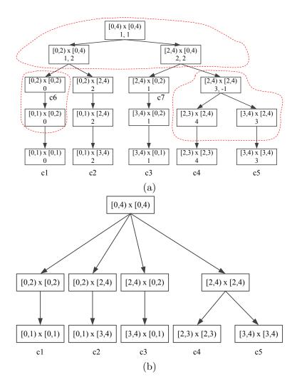
Figure 3.5: (a) Redraw the previous cbp-tree in Figure 3.3(b) with the dashed lines grouping the CCPs into QCPs, and (b) the new representation with the QCP operations.
