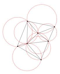
Figure 2.7: An example of a Delaunay triangulation, with the circumcircles of triangles drawn with dashed lines.
