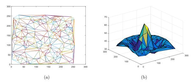
Figure 2.14: An example of mesh model of image. (a) The original triangulation of the image domain and (b) 2.5-D triangle mesh model with the associate piecewise-linear function.
