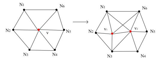
Figure 2.12: An example of vertex split leading to invalid triangulation. (a) Before vertex split and (b) after vertex split.
