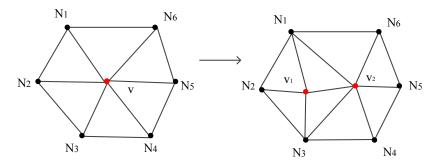
Figure 3.28: An example of vertex split. Vertex v is split into two new vertices  $v_1$  and  $v_2$ .
