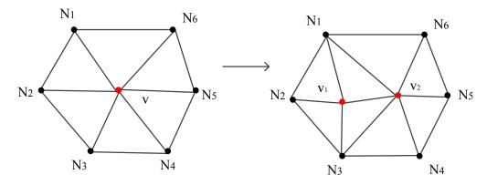
Figure 3.7: An example of vertex split. Vertex v is split into two new vertices  $v_1$  and  $v_2$ .
