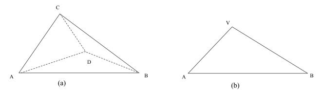
Figure 3.29: A simple 3-D triangle mesh. (a) Original mesh with four vertices (A, B, C, and D) and three faces ( $\triangle ABC$ ,  $\triangle ADC$ , and  $\triangle BCD$ ), and (b) the latest version of a coarser mesh.
