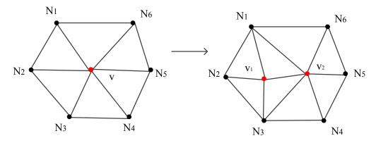
Figure 2.11: An example of vertex split. Vertex v is split into two new vertices  $v_1$  and  $v_2$ .
