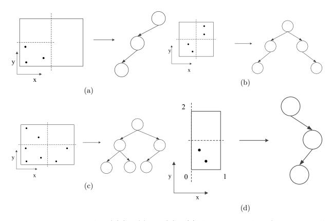
Figure 3.11: Four examples of QCP. After a QCP, (a) the actual number of nonempty cells is T = 1 and the maximum number of nonempty cells is M = 4. Similarly, (b) T = 2 and M = 4 and (c) T = 3, M = 4. (d) Since the cell bi-partitioning along *x*-axis generates a degenerate cell, so the maximum number of nonempty cells M = 2, and the actual number is T = 1.
