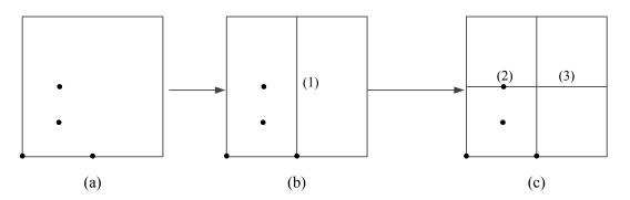
Figure 3.4: An example of a QCP containing three CCPs. (a) Original cell to split. (b) The first CCP along x-axis, and (c) the other two CCPs along y-axis.
