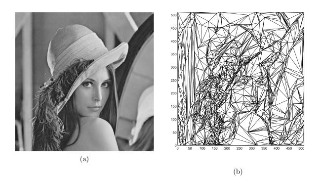
Figure 1.3: (a) An image, and (b) a set of nonuniformly sampled points with a triangulation on these points partitions the image domain into nonoverlapping triangles.
