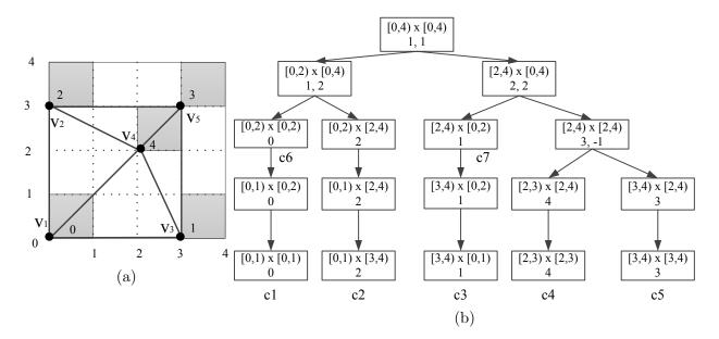
Figure 3.3: An example of a cbp-tree. (a) A mesh with five sample points, and (b) its corresponding cbp-tree representation showing only geometry and function value information.
