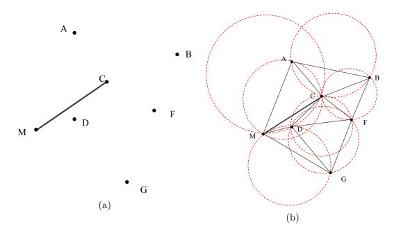
Figure 2.10: Constrained Delaunay triangulation example. (a) A PSLG (P, E) containing a set P of points (where  $P = \{A, B, C, D, F, G, M\}$ )and a set E of one segment (where  $E = \{\overline{CM}\}$ ), and (b) the constrained Delaunay triangulation T of (P, E), with the circumcircles of triangles in T drawn using dashed lines.
