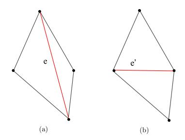
Figure 2.5: An example of an edge-flipping operation, flipping (a) edge e in one triangulation to (b) edge e' in another.
