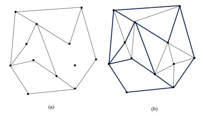
Figure 2.9: An example of (a) a PSLG and (b) a constrained triangulation of the PSLG.
