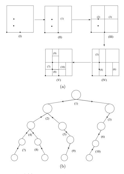
Figure 3.2: An example of (a) a recursive cell partitioning procedure, and (b) the corresponding cbp-tree structure. The labels  $\{(1), (2), \ldots, (10)\}$  have one-on-one correspondence in (a) and (b).
