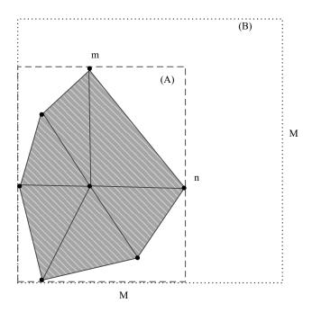
Figure 3.1: An example of root cells for different schemes. The gray area is conv(P), where P is the set of sample points. Dashed lines (A) and (B) represent the root cells under unpadded and padded schemes, respectively.
