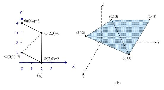
Figure 2.13: An example of a 2.5-D triangle mesh with four sample points. (a) The triangulation and its associated sampled function values, and (b) the surface obtained from piecewise-linear interpolation. Here z-axis represents the function value of  $\tilde{\phi}$ .
