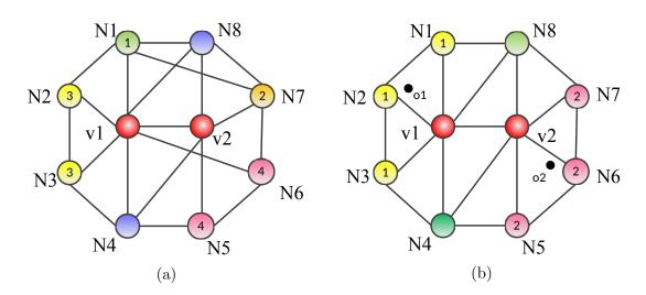
Figure 3.10: Two examples of nonpivots partitioning. In (a), four segments are generated for the nonpivots. In (b), two segments are generated for nonpivots with the centroids of the segments denoted as  $o_1$  and  $o_2$ .
