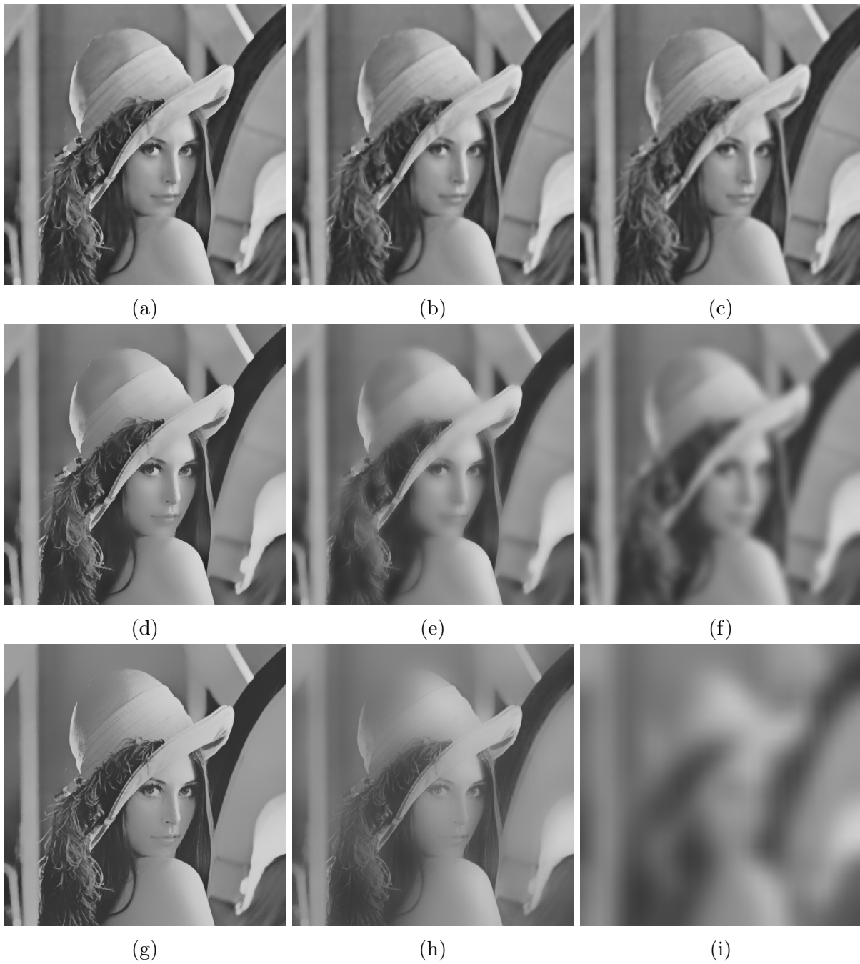
Figure 2.1: Effect of the space ( \sigma_s ) and range ( \sigma_r ) parameters on the output of the bilateral filter. The filter approximates a Gaussian for \sigma_r \approx \infty .
