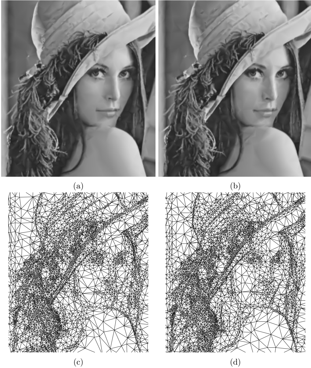
Figure 4.3: Part of the image approximation obtained for the lena image at a sampling density of 2% with the proposed (a) IID1 method (32.10 dB), and (b) the ID1 method (32.15 dB), and (c) and (d) their corresponding triangulations.
