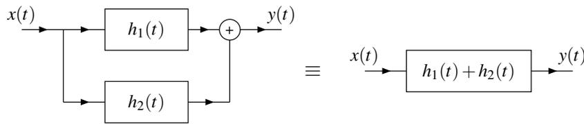
Figure 3.9: Parallel interconnection of continuous-time LTI systems.
