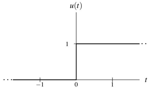
Figure 2.15: Unit-step function.
