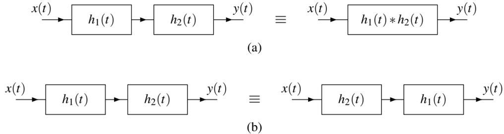
Figure 3.8: Series interconnection of continuous-time LTI systems.
