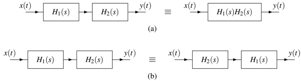
Figure 6.17: System function and series-interconnection of LTI systems.
