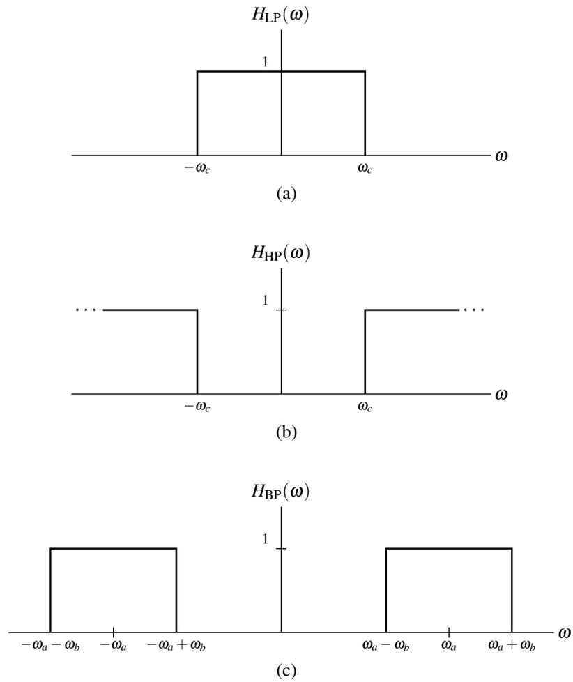
Figure 5.18: Frequency responses of systems from example.
