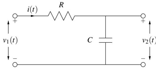
Figure 6.16: Simple RC network.
