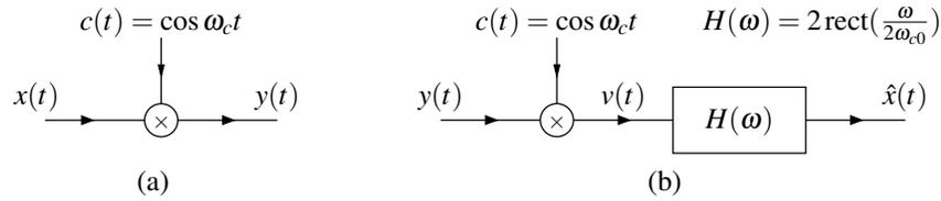
Figure 5.32: DSB/SC amplitude modulation system. (a) Transmitter and (b) receiver.
