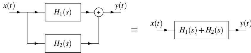
Figure 6.18: System function and parallel-interconnection of LTI systems.
