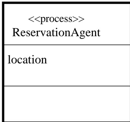
An **Active Object** is an object that owns a process or thread and can initiate control activity.
