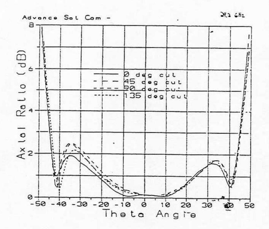
Figure 5: Measured axial ratio of the complete feed
