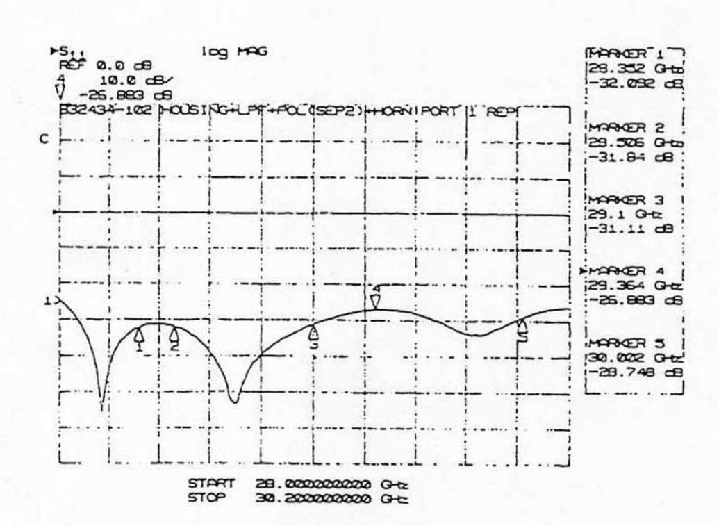
Figure 4: Return loss of the overall feed chain
