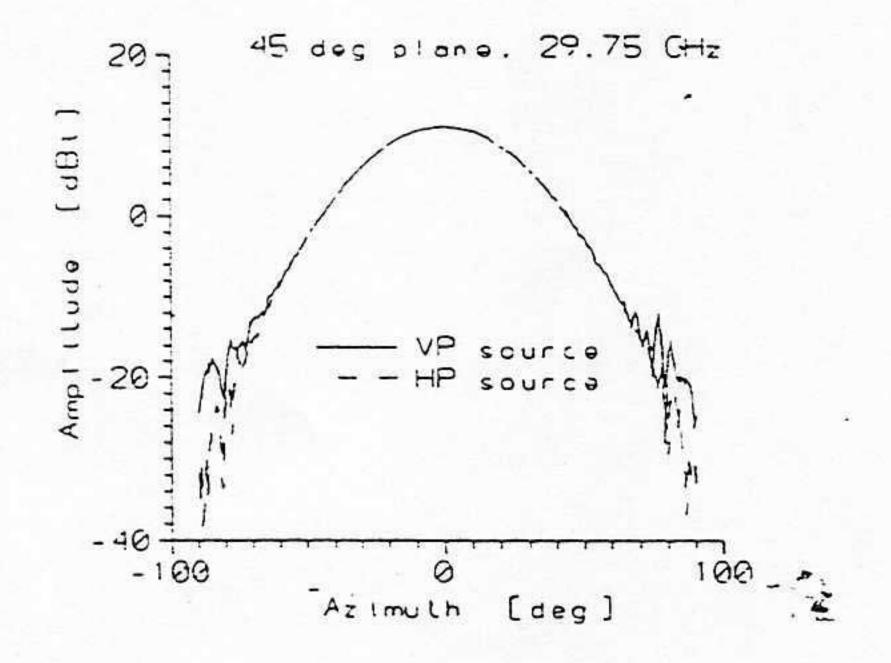
Figure 3: Radiation pattern of the feed variant 1.
