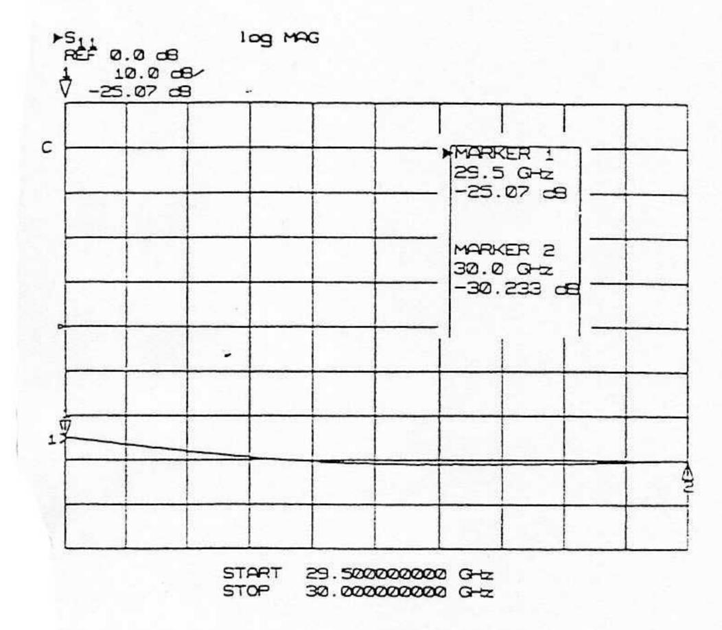
Figure 2: Return loss of the entire feed chain (design variant 1)
