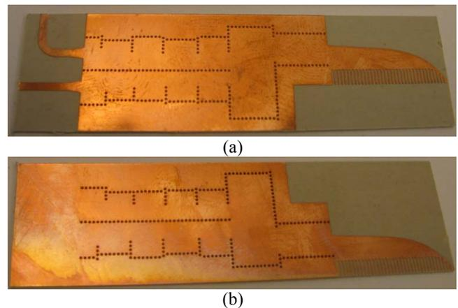
Fig. 1. Photographs of the diplexing SIW antenna system; front (a), back (b).
