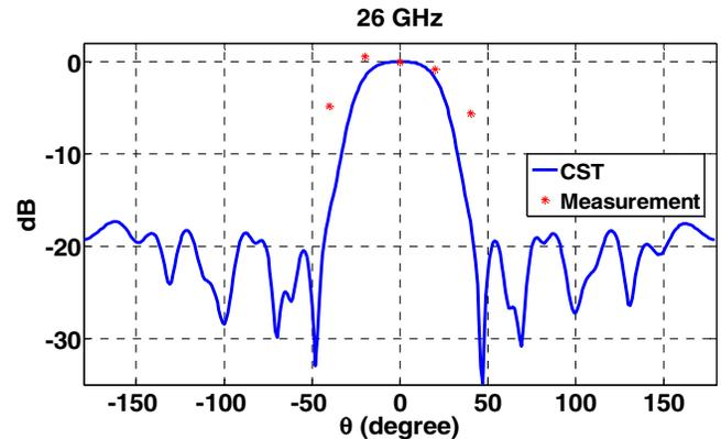
Fig. 4. Comparison between simulated (CST - solid line) and measured (asterisk) radiation patterns in the upper band at 26 GHz.
