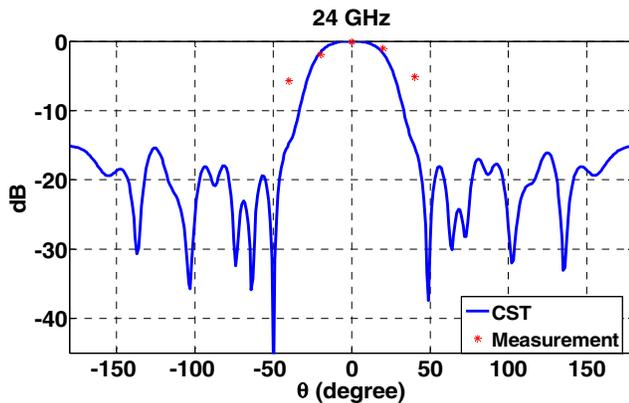
Fig. 3. Comparison between simulated (CST - solid line) and measured (asterisk) radiation patterns in the lower band at 24 GHz.
