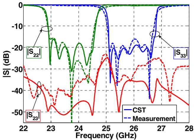
Fig. 2. Comparison between simulated (solid lines) scattering parameters with CST and measured data (dashed lines).
