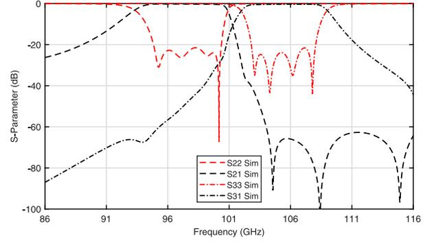
Fig. 8.  $S$ -parameters of the simulated mixed-inverter diplexer (conductivity of brass taken as  $1.59 \times 10^7$  S/m).
