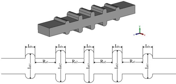
Fig. 3. Perspective view of the admittance-inverter filter's vacuum shell and its corresponding dimensions;  $R_{a1} = 1.695$  mm,  $R_{a2} = 1.524$  mm,  $I_{alx} = 0.800$  mm,  $I_{ah1} = 2.032$  mm,  $I_{ah2} = 2.578$  mm, and  $I_{ah3} = 2.680$  mm.
