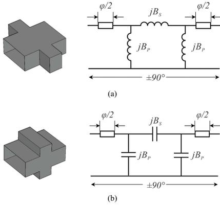
Fig. 2. Waveguide admittance inverters and their corresponding circuit topologies. (a) Inductive stub. (b) Capacitive stub.
