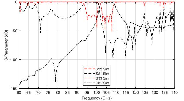
Fig. 9. Wideband spurious performance of the simulated mixed-inverter diplexer (conductivity of brass taken as  $1.59 \times 10^7$  S/m).
