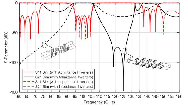
Fig. 5. Wideband spurious performance of the simulated admittance-inverter filter with comparison to an impedance-inverter filter with similar specifications (conductivity of copper taken as  $5.8 \times 10^7$  S/m).
