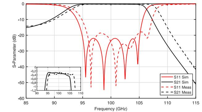
Fig. 11. Simulated versus measured  $S$ -parameters of the 3-D-printed admittance-inverter filter. The inset shows a close-up view of the insertion loss (equivalent conductivity of copper taken as  $4.2 \times 10^6$  S/m).
