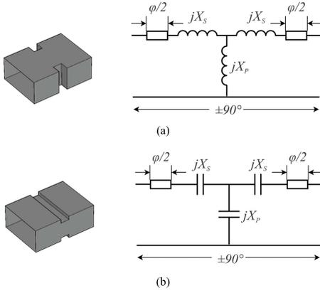
Fig. 6. Waveguide impedance inverters and their corresponding circuit topologies. (a) Inductive iris. (b) Capacitive iris.
