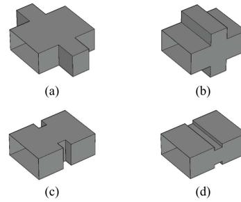
Fig. 1. Basic forms of waveguide inverters. (a) Inductive stub. (b) Capacitive stub. (c) Inductive iris. (d) Capacitive iris.
