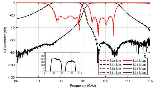
Fig. 12. Simulated versus measured  $S$ -parameters of the high-precision milled mixed-inverter diplexer. The inset shows a close-up view of the insertion loss in the lower and upper passbands (equivalent conductivity of brass taken as  $7.7 \times 10^6$  S/m).
