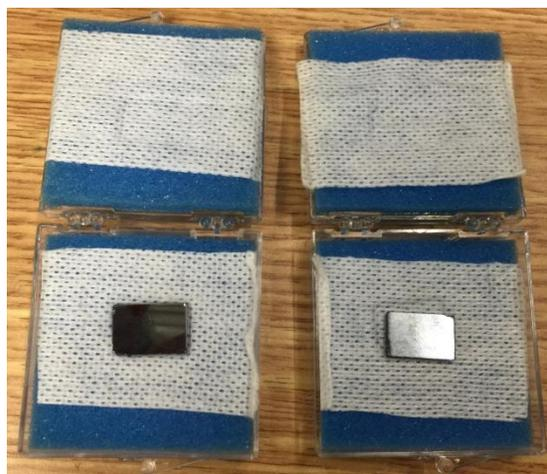
**Figure 1: CZT samples Detectors 6 and 8 used in characterization analysis**
