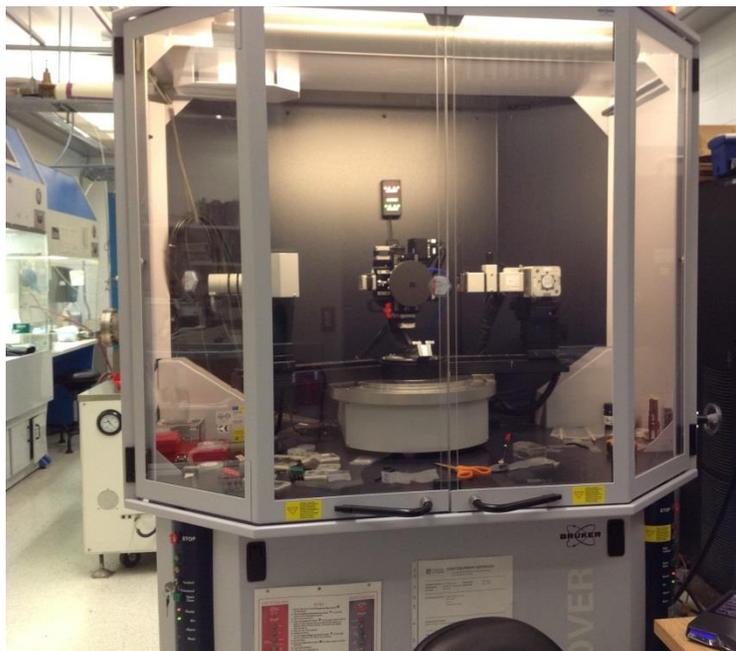
**Figure 3: Bruker D8 Discover diffractometer system analyzing a CZT sample**
