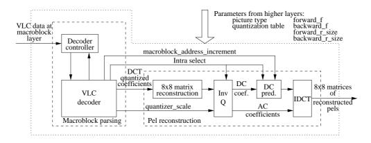
Figure 1. Macroblock parsing and pel reconstruction module – adapted from [5].
