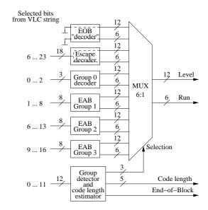
Figure 3. The VLD implementation on FPGA.
