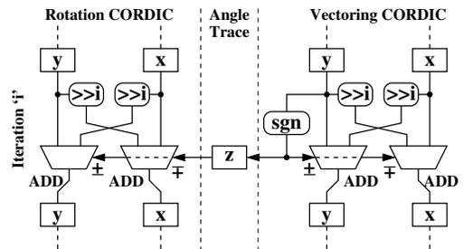
Fig. 2. A CORDIC pipeline stage and the angle trace.
