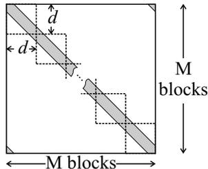
**Fig. 1.** Channel State Matrix Decomposition (gray regions contain values with largest magnitudes) – adapted from [2, 3].
