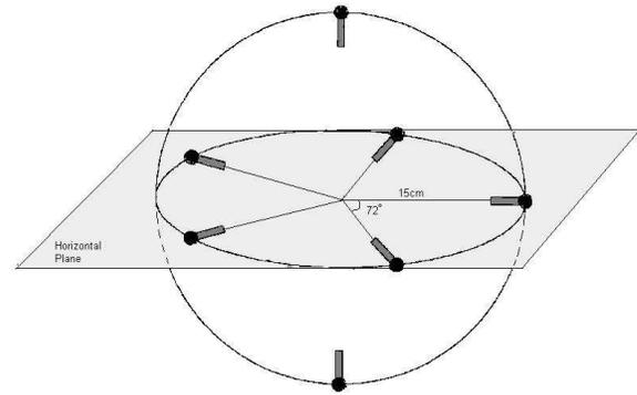
Fig. 1. Microphone Array
