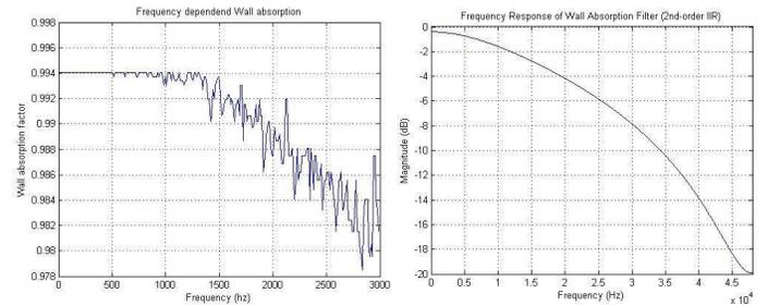
Fig. 4. 2nd-order IIR approximation of wall filter
