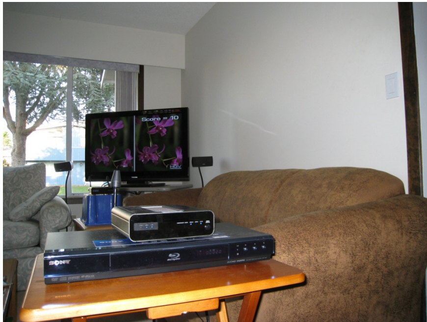
Figure 14. Test setup for the ZeroWire HDMI video test. Both the server and the client were placed 90 cm above the ground.
